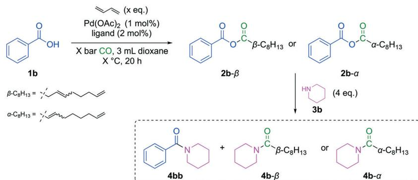
Fig. 8 Carbonylative telomerization of 1,3-butadiene with benzoic acid (**1b**) for the synthesis of mixed anhydrides (**2b**) prior to optimization and subsequent derivatization yielding amides for quantification.
