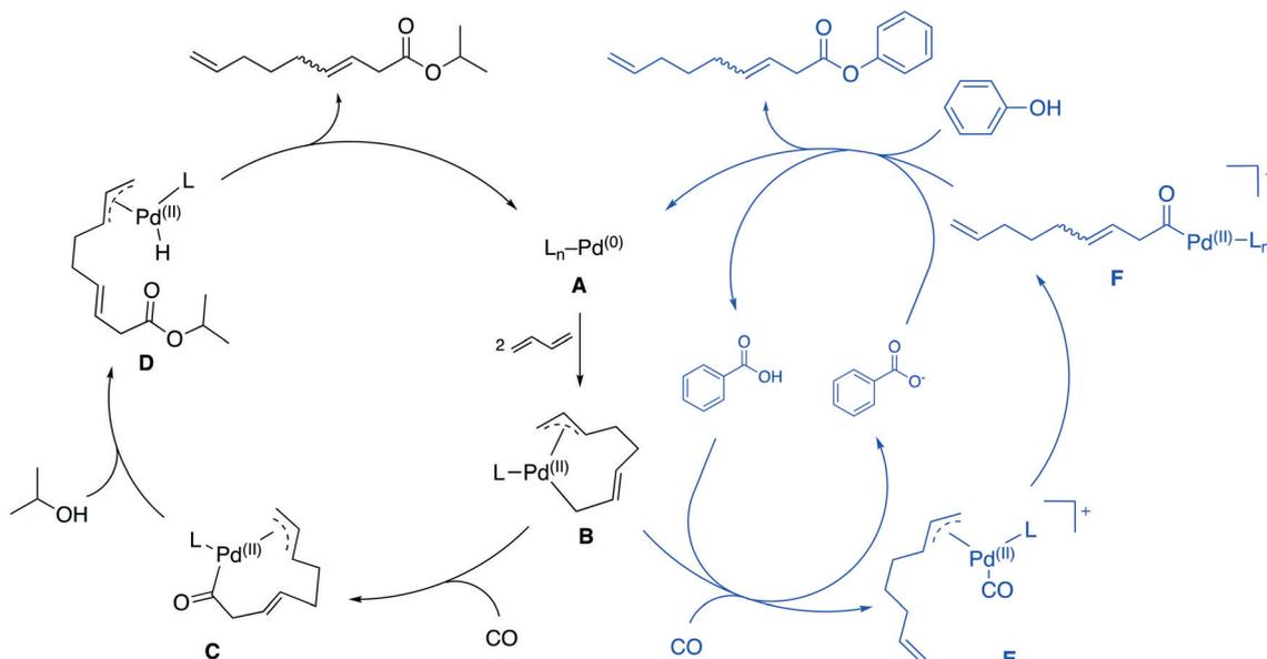
Fig. 2 Catalytic cycles proposed for the carboxytelomerization proposed by Knifton (left),<sup>3</sup> and Sauthier (right).<sup>10</sup>
