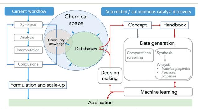
Fig. 6 Feedback loops in current (left, blue arrows) and automated/autonomous (right, red arrows) catalyst discovery.
