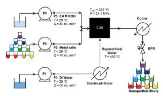
Fig. 5 Flow chart for the synthesis of a Ba<sub>x</sub>Sr<sub>v</sub>Ca<sub>z</sub>TiO<sub>3</sub> sample nanoparticle library of candidate ORR catalysts composed of 66 materials. P1 is pump 1, P2 is pump 2, and P3 is pump 3. BPR stands for back-pressure regulator and CJM stands for confined jet mixer. Reprinted with permission from A. R. Groves, T. E. Ashton, J. A. Darr, ACS Combinatorial Science, 2020, 22, 750-756. Copyright 2022 American Chemical Society
