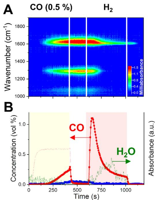
Fig. 5 Dynamic evolution of surface species elucidated by *operando* DRIFTS (A) during CO-CCR performed at  $350\text{ }^\circ\text{C}$ . Outlet gas composition (B) was obtained from averaging 5 cycles. CO blank signal (dotted line) obtained as average of 2 CCR cycles during a blank experiment at room temperature.
