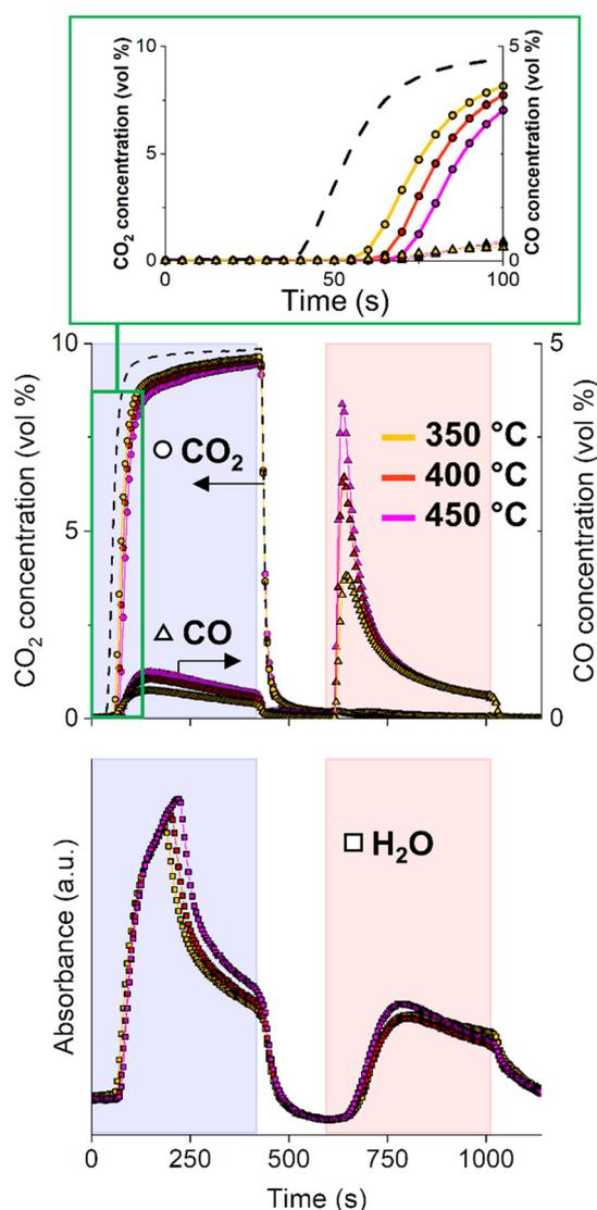
**Fig. 2** Outlet gas concentrations of CO<sub>2</sub> (o) and CO (Δ) and signal of H<sub>2</sub>O (□) during CCR performed at 350 °C (yellow profiles), 400 °C (red profiles), 450 °C (magenta profiles). Results are averaged of 18 CCR cycles. CO<sub>2</sub> blank signal (dotted line) obtained as average of 2 CCR cycles during blank experiment at room temperature.
