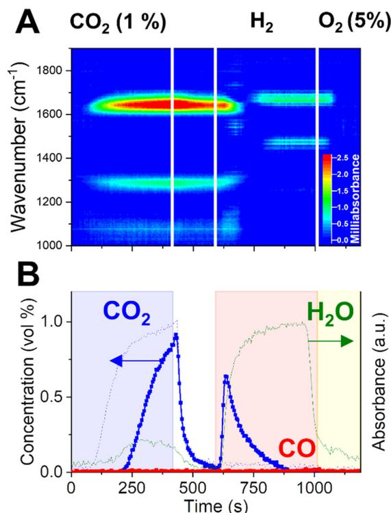
Fig. 6 Dynamic evolution of surface species elucidated by *operando* DRIFTS (A) during CCR performed at 350 °C with substitution of last He gas phase with O<sub>2</sub> (5% in He). Outlet gas composition (B) was obtained from averaging 5 cycles at 350 °C. CO<sub>2</sub> blank signal (dotted line) obtained as average of 2 CCR cycles during a blank experiment at room temperature.
