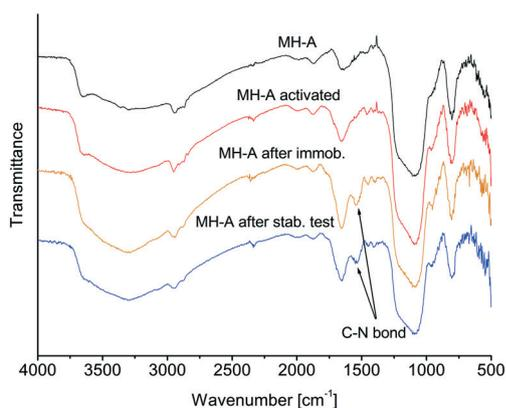
**Fig. 5** FTIR spectra of silica monoliths functionalized with amino groups (black) and subsequently activated by glutaraldehyde (red). Orange and blue line are for *AtHNL* immobilized on silica monolith respectively just after immobilization (orange) and after stability test (blue).
