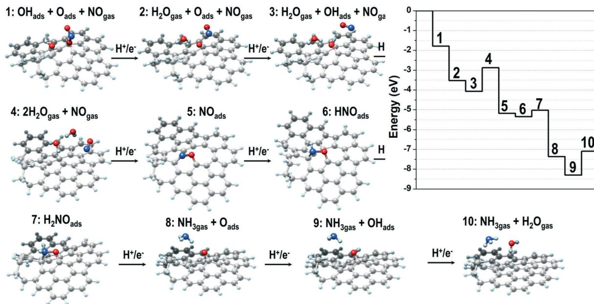
Fig. 6 Energy profile of the  $\text{NO}_3\text{RR}$  mechanism leading to the formation of  $\text{NH}_3$  and three water molecules and the corresponding configurations. These were obtained through energy minimizations at the QC level (using a reduced model system terminated with hydrogen atoms). C gray, N blue, O red, H light blue. Note that the first step is the spontaneous dissociation of  $\text{HNO}_3$  at the carbon surface.
