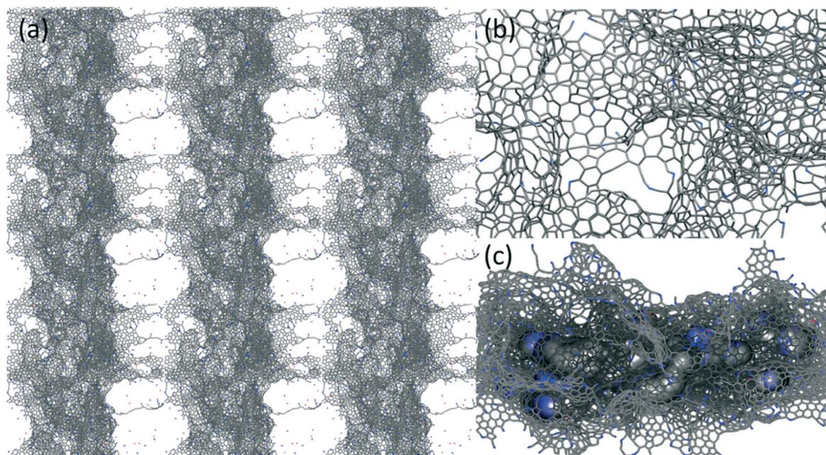
**Fig. 3** (a) The final carbonized-N-doped atomistic configuration obtained through RMD (periodic replica), (b) graphitic-like structure with N at the edges of the pores, and (c) identification of the tunnels and cavities by CAVER's sphere filling (stick models and spheres colored according to the atom type: C gray, O red, N blue).
