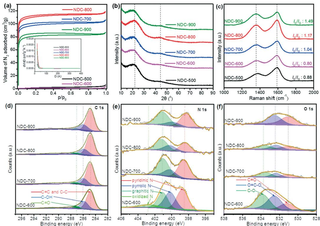
Fig. 2 (a)  $N_2$  adsorption-desorption isotherms, (b) PXRD patterns and (c) Raman spectra of NDC-500, NDC-600, NDC-700, NDC-800 and NDC-900 materials; XPS (d) C 1s, (e) N 1s and (f) O 1s spectra of NDC-600, NDC-700, NDC-800 and NDC-900 materials.
