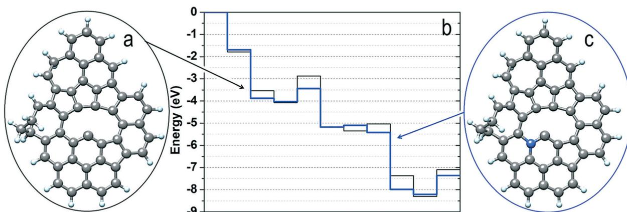
Fig. 7 (a) Structure of the bare defect sampled as the catalytic site in the mechanism shown in Fig. 6; (b) energy profiles for the  $\text{NO}_3\text{RR}$  mechanism characterizing sites (a) and (c); (c) same structure of panel (a) where one C atom next to the defect border has been replaced with a nitrogen atom.
