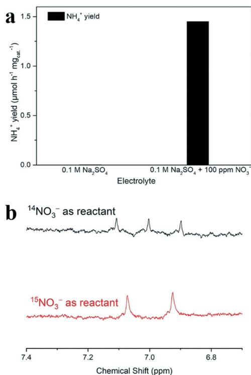
Fig. 5 (a)  $\text{NH}_4^+$  yield of NDC-800 in 0.1 M  $\text{Na}_2\text{SO}_4$  electrolyte with and without 100 ppm  $\text{NO}_3^-$  for 2 h CA; (b)  $^1\text{H}$  NMR spectra of the electrolyte after the electrocatalytic  $\text{NO}_3\text{RR}$  using  $^{15}\text{NO}_3^-$  and  $^{14}\text{NO}_3^-$  as the nitrogen sources.
