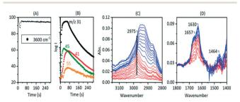
Fig. 15 An 8  $\mu$ L pulse of CH<sub>3</sub>OH at 673 K on HSAPO-34. (A)  $\nu$ (OH) intensity *versus* time. (B) Corresponding MS traces (m/z=31 measures methanol; m/z=41, propene with a contribution from fragmentation of DME, m/z=45, DME; m/z=55, butene). (C and D) Difference infrared spectra at 2 s intervals. Red: from 2 s to 20 s. Blue: from 20 to 40 s.
