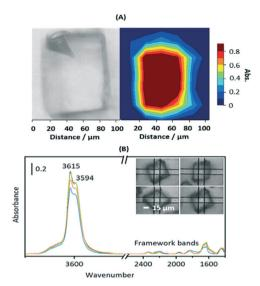
Fig. 1 (A) Optical image and distribution of Brønsted acid sites within one crystal (integrated OH intensity between 3650 and 3550 cm<sup>-1</sup> and normalised to 1). (B) FTIR spectra of four dehydrated HSAPO-34 crystals of similar size (inset), measured with a 15  $\times$  15  $\mu$ m<sup>2</sup> aperture. Note that the exact frequencies are temperature dependent; the spectra shown were measured at 623 K.
