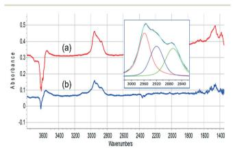
Fig. 8 Infrared difference spectra measured (a) after exposure of SAPO-34 crystal to 2 8  $\mu L$  pulses of methanol at 573 K and flushing in nitrogen; (b) after exposure of SAPO-34 crystal to propene at 473 K and flushing in nitrogen. The insert shows a curve fit of spectrum (a) in the n(CH) region.
