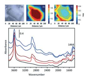
Fig. 13 (a) Optical image of a SAPO-34 crystal exposed to DME at 573 K for 1000 s then flushed with nitrogen for 10 min. (b) Maps of the v(OH) intensity at 3610 cm<sup>-1</sup> and (c) the v(CH) intensity at 2955 cm<sup>-1</sup> (baseline corrected) from the same crystal. Lower traces: selected unsubtracted spectra from the centre of the crystal (bottom red) and the outer rim (top blue). The black trace is the dehydrated zeolite before reaction.
