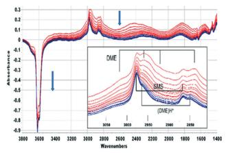
Fig. 4 Difference spectra shown at 40 s intervals from 60 s after injecting an 8 μL pulse of CH<sub>3</sub>OH into a SAPO-34 crystal at 523 K. The spectrum of the dehydrated SAPO-34 crystal has been subtracted from each spectrum. Colour change from red to blue after 420 s. The inset shows an expansion of the  $\nu(CH)$  region, showing bands due to hydrogen bonded dimethylether, surface methoxy species and protonated.
