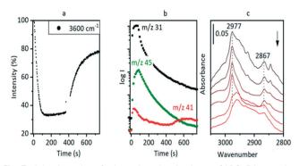
Fig. 7 Injection of an 8 µL methanol pulse into a SAPO-34 crystal at 573 K. (A) Intensity of acid site v(OH) band relative to dehydrated crystal following injection at t = 0. (B) MS analysis of effluent gas. m/z = 31measures methanol, m/z = 45 measures DME and m/z - 41 measures propene, with an initial contribution from fragmentation of DME. (c) Selected spectra in the v(CH) region (top to bottom) at t = 60 s, 120 s, 300 s, 366 s, 550 s, 750 s. Bands marked are those of SMS.
