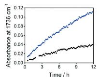
Fig. 6 Plots of absorbance vs. time for v(C=O) of MeOAc during carbonylation experiments using 3 (blue) or Bu<sub>4</sub>N[Rh(CO)<sub>2</sub>I<sub>2</sub>] (grey) (120 °C, 10 bar CO, 0.8 M Mel in MeOH).
