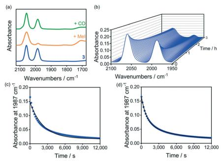
Fig. 4 (a) IR spectra (KBr disc, v(CO) region) of pristine 3 (blue), after soaking in MeI (orange) and after exposure to CO (green), (b) series of IR spectra (v(CO) region) during reaction of 3 with 1 M MeI in CH<sub>2</sub>Cl<sub>2</sub> (25 °C) and decay of IR absorption at 1987 cm<sup>-1</sup> during this reaction with (c) single exponential curve fit, and (d) double exponential curve fit.
