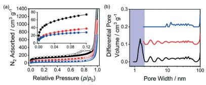
Fig. 2 (a) Nitrogen adsorption (filled) and desorption (open) isotherms at 77 K (offset successively by 25 cm $^3$  g $^{-1}$ ), inset shows the low relative pressure region (with no offset); (b) differential pore size distribution (offset successively by 0.1 cm $^3$  g $^{-1}$ , micropore region highlighted) of 1 (black), 2 (red) and 3 (blue).
