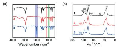
Fig. 1 (a) FTIR spectra highlighting the absorptions due to v(C-N) (green), v(C-O) (red) and v(C=O) (blue); (b) solid state <sup>13</sup>C{<sup>1</sup>H} CP/MAS NMR of materials 1 (black), 2 (red) and 3 (blue).
