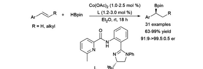
Scheme 54 Cobalt-catalysed  $\alpha$ -selective hydroborations of *trans*-1,2-disubstituted aryl alkenes.<sup>264</sup>
