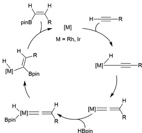
Scheme 7 Proposed mechanism for the rhodium-catalysed *trans*-hydroboration of terminal alkynes.<sup>73</sup>
