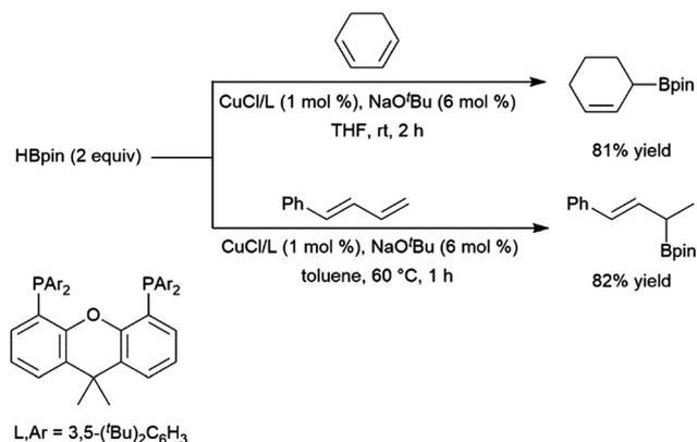
Scheme 41 Copper-catalysed hydroboration of dienes.<sup>225</sup>
