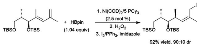
Scheme 108 Hydroboration of a diene as a step in the preparation of an intermediate in the preparation of (+)-discodermolide.<sup>221</sup>
