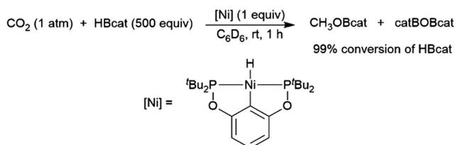
Scheme 83 Nickel-catalysed hydroboration of CO<sub>2</sub>.<sup>510</sup>
