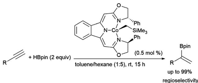
Scheme 57 Cobalt-catalysed  $\alpha$ -selective hydroboration of terminal alkynes.<sup>365</sup>
