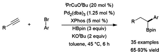
Scheme 56 One pot hydroboration-hydrocupration-cross-coupling reaction.<sup>364</sup>
