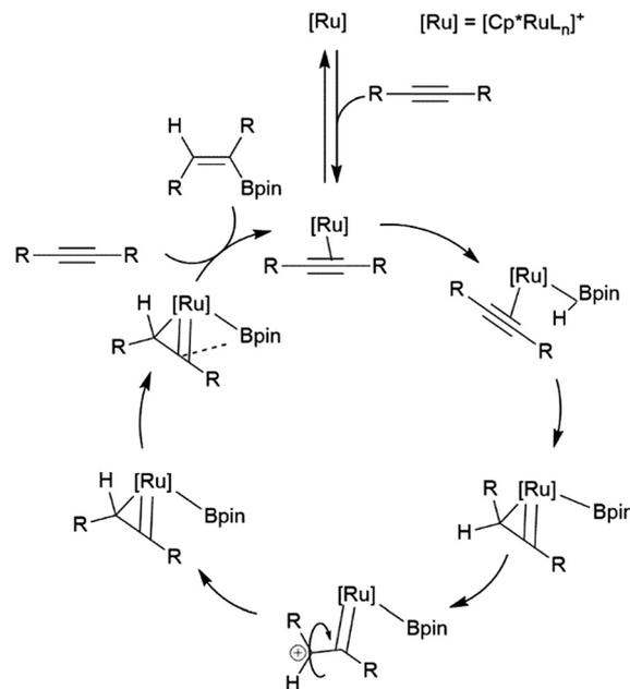
Scheme 8 Proposed mechanism for the ruthenium-catalysed *trans*-hydroboration of internal alkynes.<sup>73,74</sup>
