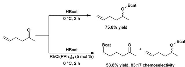
Scheme 20 Hydroboration of 5-hexen-2-one by HBcat in the absence of a catalyst (top) and using Wilkinson's catalyst (bottom).<sup>33</sup>
