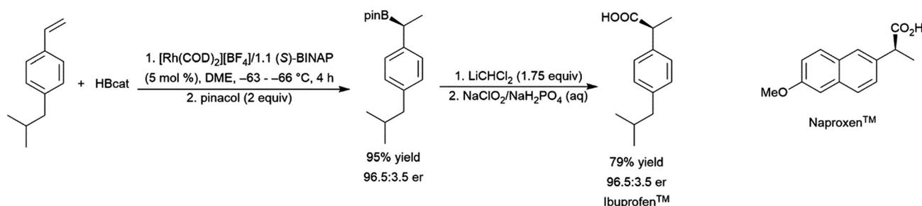
Scheme 101 Preparation of Ibuprofen™ from its corresponding styrene.<sup>571</sup>
