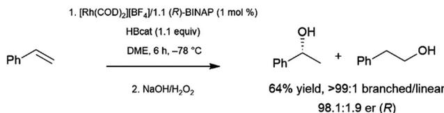
Scheme 16 Asymmetric hydroboration of styrene catalysed by a cationic rhodium(i)/BINAP catalyst.<sup>96</sup>
