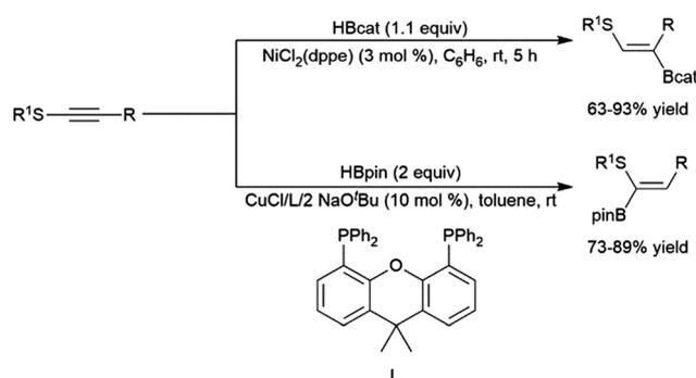
Scheme 59 Catalytic hydroborations of thioalkynes using nickel<sup>304,372</sup> (top) and copper<sup>320</sup> (bottom) catalyst systems.
