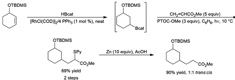
Scheme 100 Addition of methyl acrylate to an alkylboronate ester (PTOC-OMe = *N*-methoxycarbonyloxy pyridine-2-thione).<sup>155</sup>
