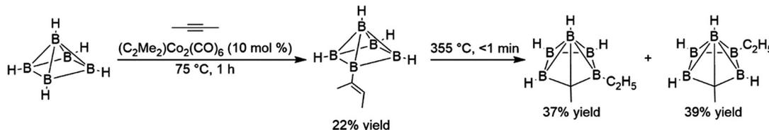
**Scheme 3** Hydroboration of dimethylacetylene using a polyhedral borane (bridging hydrides between each equatorial boron atom are excluded for clarity).<sup>8</sup>
