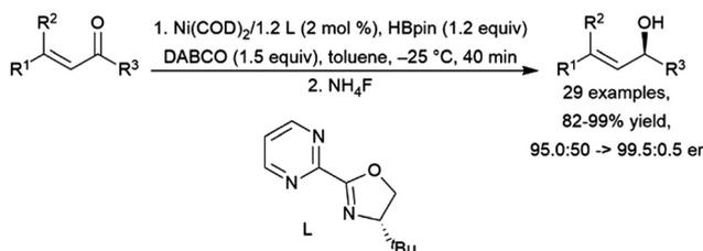
Scheme 68 Nickel-catalysed hydroboration of the ketone group of an  $\alpha,\beta$ -unsaturated ketone.<sup>461</sup>
