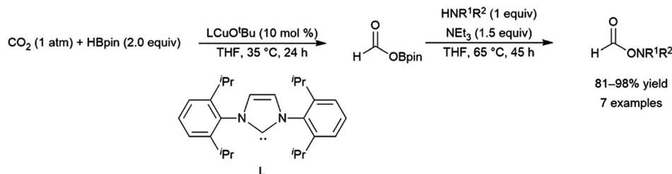
Scheme 84 One pot hydroboration–amination reaction of CO<sub>2</sub>.<sup>93</sup>
