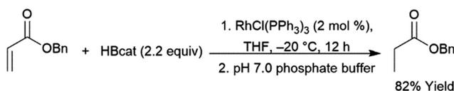
Scheme 67 Rhodium-catalysed 1,4-hydroboration of an  $\alpha,\beta$ -unsaturated ester.<sup>460</sup>
