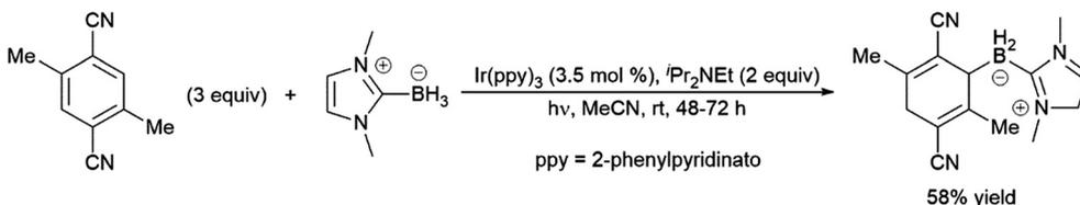
Scheme 89 Hydroboration of an electron-poor aromatic ring using a carbene–borane adduct and an iridium catalyst.<sup>564</sup>
