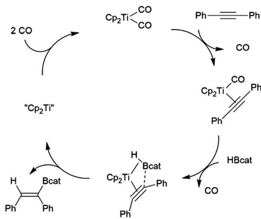
Scheme 10 Proposed mechanism for Ti(II)-catalysed hydroboration of alkynes.<sup>82</sup>
