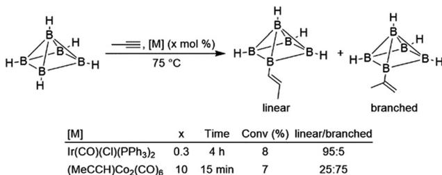
**Scheme 4** Hydroboration of propyne using a polyhedral borane (bridging hydrides between each equatorial boron atom are excluded for clarity).<sup>9</sup>
