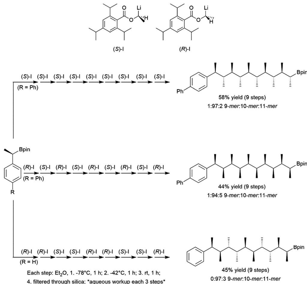
Scheme 95 Multiple homologation reaction sequence, starting with the product of a chiral hydroboration.<sup>574</sup>
