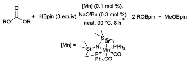
Scheme 76 Manganese-catalysed hydroboration of carbonates.<sup>476</sup>
