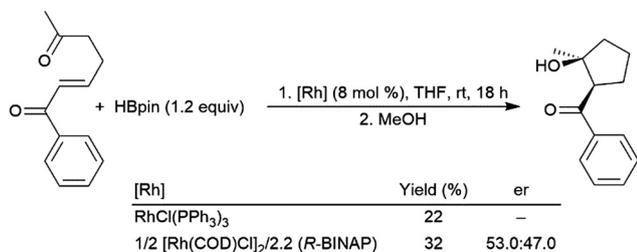
Scheme 74 Rhodium-catalysed aldol cycloaddition of an enone-ketone.<sup>474</sup>
