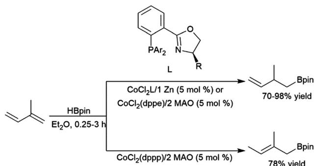
Scheme 40 Cobalt-catalysed hydroboration of dienes.<sup>223</sup>
