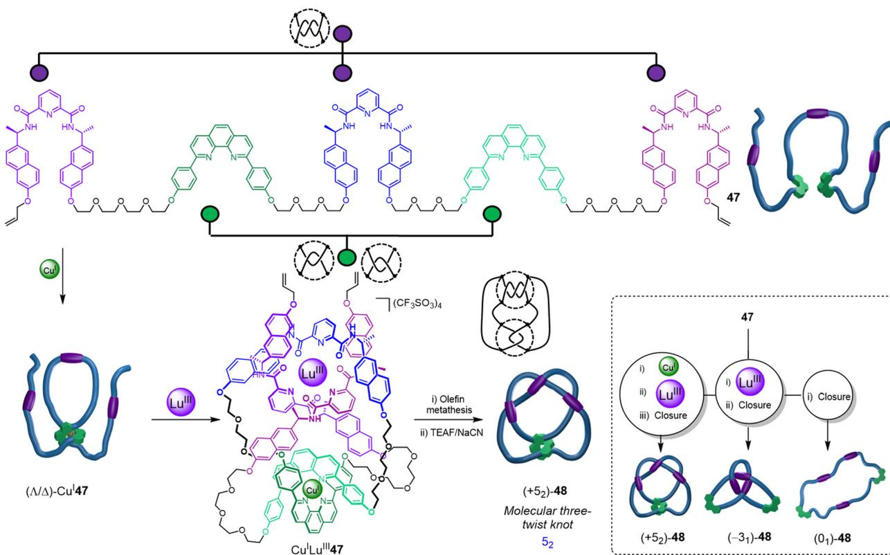
Fig. 16 Synthesis of a molecular  $5_2$  three-twist knot via stepwise folding around Cu<sup>I</sup> and Lu<sup>III</sup> templates, followed by covalent capture and demetallation. Tangles are shown next to crossing regions. Inset: A single ligand **47** forms three topoisomers:  $5_2$  knot  $(+5_2)$ -**48**, trefoil knot  $(-3_1)$ -**48** and unknot  $(0_1)$ -**48**.<sup>21</sup>
