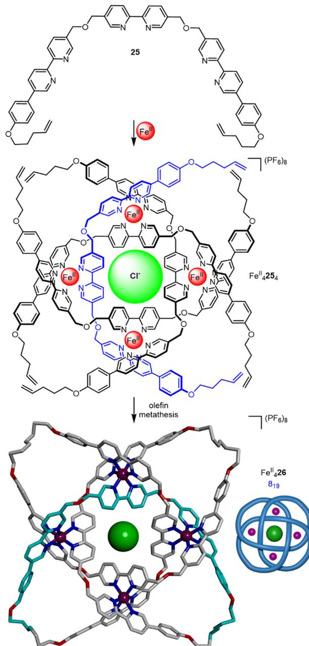
Fig. 9 Synthesis of  $8_{19}$  knot  $\text{Fe}_4^{II}26$  via braiding of three ligand strands.<sup>59</sup>
