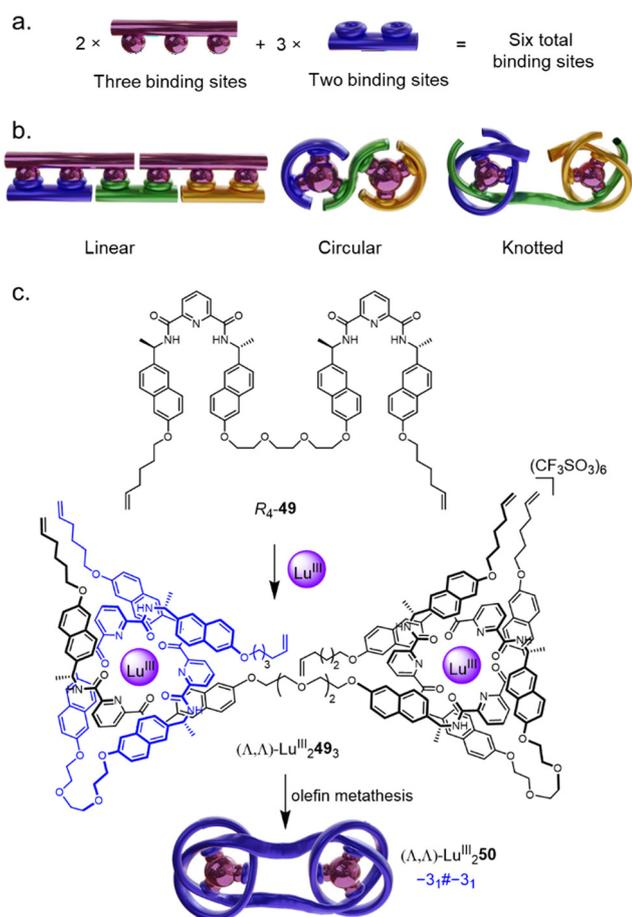
Fig. 17 (a) The Vernier template approach to increase the complexity of a system by targeted coordinative mismatch.<sup>83</sup> (b) The Vernier template approach as applied to linear, circular, and knotted systems in a 2 : 3 ratio.<sup>84</sup> (c) Synthesis of granny knot (Λ,Λ)-Lu<sup>III</sup><sub>2</sub><sup>50</sup> by Vernier template synthesis.<sup>27</sup>
