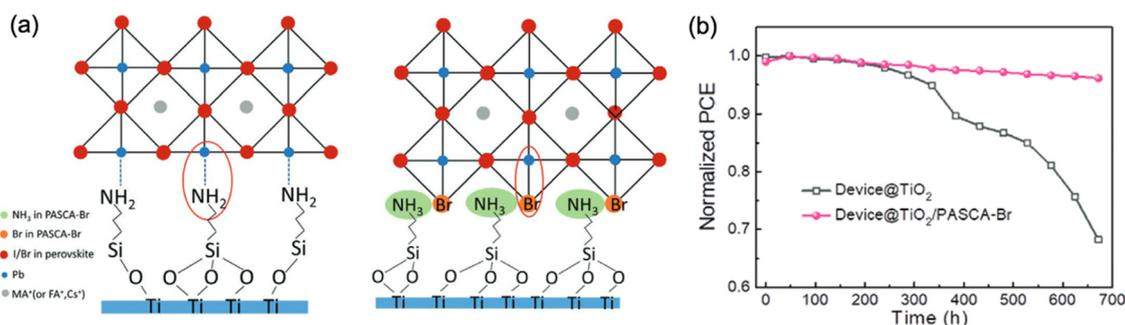
Fig. 15 (a) Lattice structure of APTES and PASCA-Br modified interfaces. (b) Stability of the devices with and without PASCA-Br modification after ageing for 1 month. Reprinted with permission<sup>100</sup> Copyright 2020, Wiley-VCH.
