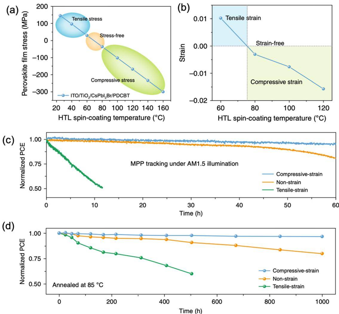
Fig. 16 (a) Calculated and (b) measured CsPbI<sub>2</sub>Br perovskite film stress variation under different spin-coating temperature of PDCBT. Stability of the devices with compressive-strain, non-strain and tensile-strain under (c) MPP tracking with AM1.5G illumination and (d) annealing temperature at 85 °C. Reprinted with permission,<sup>46</sup> Copyright 2020, Springer Nature.
