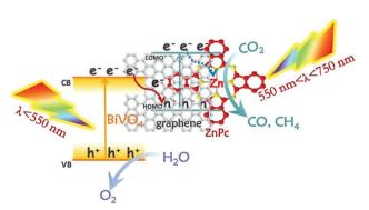
Fig. 78 Graphene-modulated ZnPc/BiVO<sub>4</sub> Z-scheme heterojunction. Reproduced from ref. 329, with permission from Royal Society of Chemistry, Copyright 2020.
