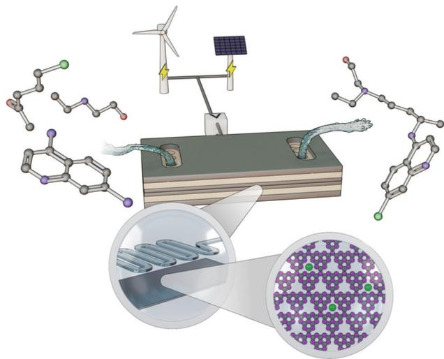
**Fig. 3** Schematic showing the electrocatalytic conversion of simpler building block molecules into value-added active pharmaceutical ingredients (in this case, hydroxychloroquine), using a single-atom catalyst incorporated within a microflow device and powered through renewable electricity.
