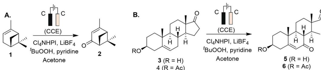
**Scheme 1** Electrochemical allylic oxidation on a 100 g scale, using inexpensive graphite plate electrodes in an open-air beaker, and LiBF<sub>4</sub> as supporting electrolyte: (A)  $\alpha$ -pinene to verbenone conversion, (B) sterol product and its acetate (CCE: constant current electrolysis).
