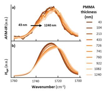
**Fig. 4** (a) Measured and (b) calculated AFM-IR spectra obtained with TIR illumination and p-polarized light for the strong carbonyl absorption for a PMMA wedge of variable thickness deposited on a ZnSe substrate. Adapted with permission from G. Ramer *et al.*, *Anal. Chem.*, 2017, **89**, 13524–13531. Copyright (2017) American Chemical Society.<sup>15</sup>
