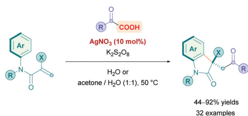
Scheme 55 Kochi conditions used for an interrupted Giese where the conjugate addition intermediate is trapped by an arene for cyclisation.
