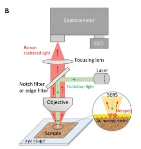
Fig. 1 (A) Schematic representation of an AFM system; (B) schematic representation of a Raman spectrometer. In a SERS configuration, the LSPR of metal (Au here) nanoparticles in contact with the sample is excited resonantly
