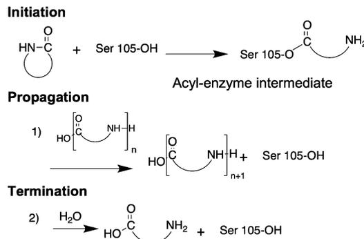
Fig. 5 Mechanism of enzyme catalyzed ring opening polymerization.
