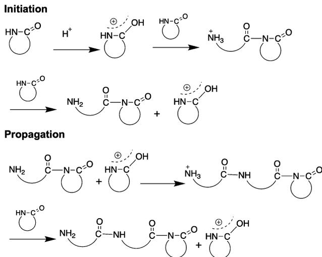
Fig. 6 Mechanism of cationic ring opening polymerization.
