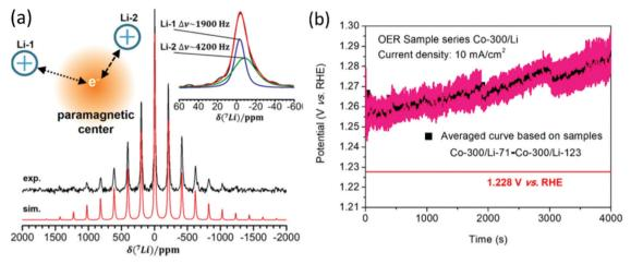
Fig. 92 (a).7Li MAS NMR spectrum of (as-prepared) Co-300/Li recorded at 11.7 T and a MAS frequency of 25.0 kHz, showing a broad, asymmetric spinning sideband pattern characteristic of a strong electron-Li dipolar interaction. (b). Averaged chronopotentiometry curve based on 53 samples of the sample series Co-300/Li (blacksquares) with standard error bars (magenta). Reproduced with permission from ref. 1324. Copyright American Chemical Society 2018.
