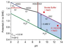
**Fig. 150** Pourbaix diagram for electrolysis of 0.5 M NaCl. The electrode potential for OER is included as well, assuming oxygen partial pressure of 0.021 MPa. The red square points show the operating potentials (vs. SHE) after 1 h constant current density of 10 mA cm $^{-2}$  with NiFe LDH catalyst in 0.1 M KOH + 0.5 M NaCl (pH 13) and 0.3 M borate buffer + 0.5 M NaCl (pH 9.2) electrolyte. Reproduced with permission from ref. 1864 Copyright Wiley 2016.
