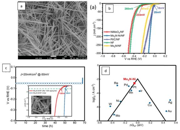
Fig. 116 SEM image of  $Mo_2N-Ni/NF$ (a). LSV curves with iR correction in 1 M KOH (b). LSV curves of  $Mo_2N-Ni/NF$  before and after a 100 h aging test, and the SEM image of  $Mo_2N-Ni/NF$  after a 100 h aging test (c). Volcano plot of  $i_0$  as a function of  $\Delta G_H^*$  for  $Mo_2N-Ni$  and some typical reported electrocatalysts (d). Reproduced with permission from ref. 1458. Copyright American Chemical Society 2020.
