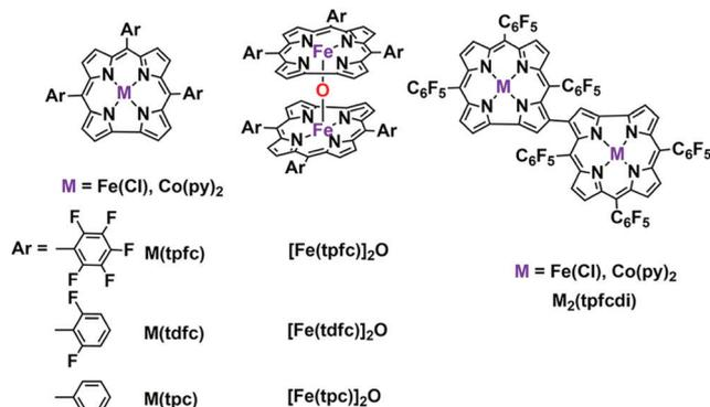
**Fig. 127** Iron and Cobalt Metalloporphyrins tested and compared as WOCs in the study presented by Sinha *et al.*<sup>1577</sup> Reprinted with permission from ref. 1577 Copyright 2020. American Chemical Society.
