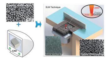
Fig. 89 Schematic representation of the fabrication process of the CESS Reproduced with permission from ref. 1299. Copyright RSC 2017.
