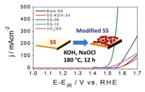
Fig. 87 Fe<sub>2</sub>O<sub>3</sub>//NiO nanocrystals were formed on the surface of corroded AISI 304 steel and significantly improved the capability of the material to act as an OER electrode. Reproduced with permission from ref. 1285 Copyright American Chemical Society 2017
