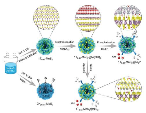
Fig. 82 Schematics of the  $1T_{0.72}$ -MoS<sub>2</sub>@NiS<sub>2</sub> and  $1T_{0.81}$ -MoS<sub>2</sub>@Ni<sub>2</sub>P synthesis steps. Reproduced with permission from ref. 1185 Copyright Nature Publishing 2021.
