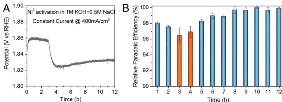
**Fig. 152** Cation-selective layer generation during anodic activation (A) chronopotentiometry plot whilst second activation step in salty electrolyte. (B) The associated OER relative faradaic efficiency plots for O<sub>2</sub> production. Reproduced with permission from ref. 1857 Copyright PNAS 2019.
