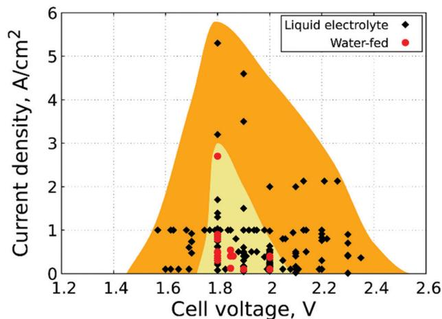
Fig. 12 Performance summary of AEMWEs: comparison of current densities achieved at cell voltages in the 1.5–2.4 V range, extracted from different polarisation curves with different feed types. Yellow and orange areas represent AEMWE performance data with (KOH addition) and without liquid electrolyte (pure water). Operating temperature ranges from 22 to 90 °C. Main design parameters, operating conditions and underlying sources are provided in Tables S3 and S4 (ESI $^{\dagger}$ ).
