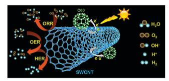
Fig. 99 Illustration of charge-transfer process and ORR/OER/HER on C<sub>60</sub>-SWCNTs. Reproduced with permission from ref. 1405. Copyright American Chemical Society 2019.
