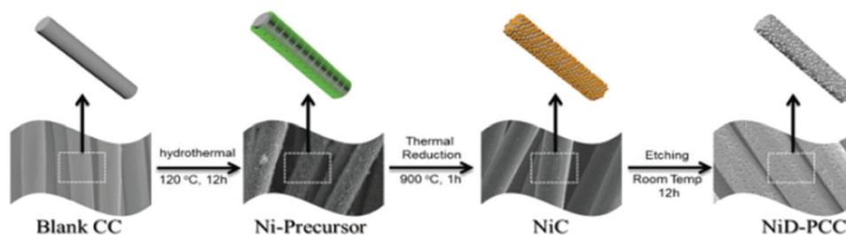
Fig. 96 Schematic illustration of the synthesis of the monolith 3D NiD-PCC. Reproduced with permission from ref. 1377. Copyright 2010 Royal Society of Chemistry (RSC).
