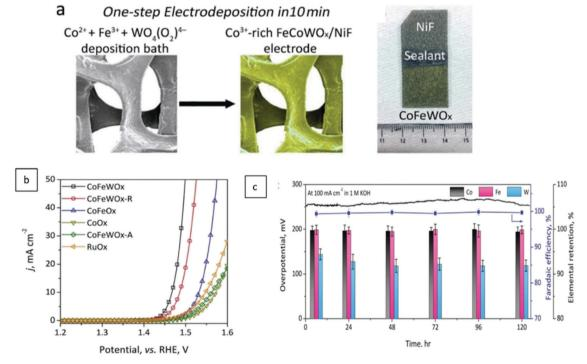
Fig. 113 A schematic illustration of the electrodeposition of CoFeWOx on NFs (a), In 1.0 M KOH aqueous electrolyte, catalytic output of catalysts deposited on glassy carbon electrodes (GCEs) for OER in three-electron configuration (b). The electrolyser was tested for stability at 100 mA cm<sup>-2</sup> in 1.0 M KOH electrolyte. During electrolysis, the elemental preservation of Co, Fe, and W in FeCoWOx/NiF (c). Reproduced with permission from ref. 1456. Copyright Wiley 2020
