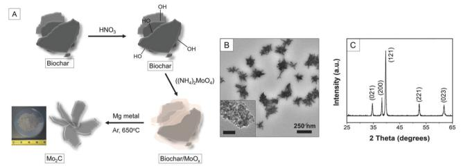
Fig. 63 (A) Schematic representation of synthesis of Mo<sub>2</sub>C nanostructures. (B) TEM image (inset: scale bar = 25 nm) and (C) the powder XRD pattern of Mo<sub>2</sub>C derived from biochar. Reproduced with permission from ref. 1002. Copyright Wiley 2018
