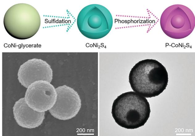
Fig. 84 Schematic presentation of the synthesis steps leading to P-CoNi<sub>2</sub>S<sub>4</sub> YSS particles and TEM images of these particles. Reproduced with permission from ref. 1179 Copyright Wiley 2021.
