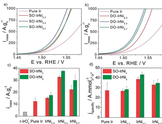
Fig. 103 (a and b) sweep voltammetry and catalytic oxygen evolution reaction (OER) activities of stepwise oxidised (SO) IrNi<sub>x</sub> and directly oxidised (DO) IrNi<sub>x</sub> core-shell nanoparticles, compared to pure Ir nanoparticles. (c) Ir mass-based activities and (d) specific activities at 0.25 V overpotential. Reproduced with permission from ref. 1429. Copyright RSC 2014.
