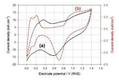
Fig. 104 (a) Volcano plots of  $j_0$  vs. M-H bond energy. (b) SEM micrographs of nano-Pt/C electrocatalysts for the HER. (c) Cyclic voltammograms measured (a) on metallic Pt in 1 M  $H_2SO_4$ ; (b) in situ at the cathode of a PEM water electrolysis cell. Reproduced with permission from ref. 1431 Copyright Elsevier 2014
