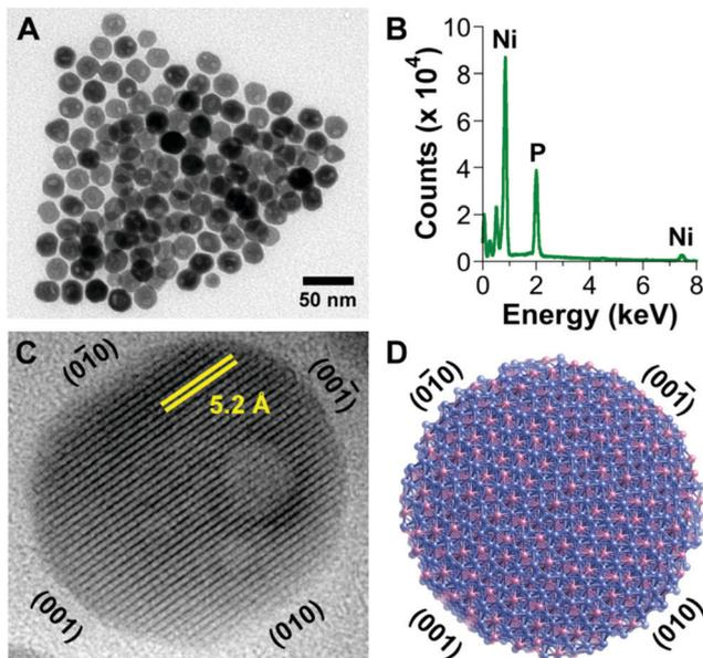
Fig. 71 (A) TEM image and (B) EDX spectrum of  $\text{Ni}_2\text{P}$  nanoparticles. (C) HRTEM image of a representative  $\text{Ni}_2\text{P}$  nanoparticle, highlighting the exposed  $\text{Ni}_2\text{P}(001)$  facet and the 5.2 Å lattice fringes that correspond to the (010) planes. (D) Proposed structural model of the  $\text{Ni}_2\text{P}$  nanoparticles. Reproduced with permission from ref. 1259 Copyright 2013 American Chemical Society.
