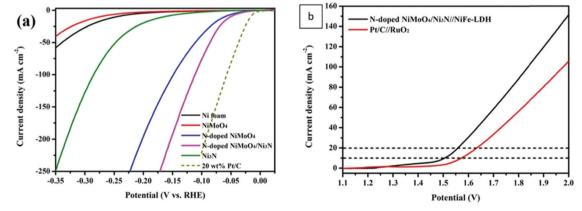
Fig. 115 Polarisation curves of Ni foam, NiMoO<sub>4</sub>, N-doped NiMoO<sub>4</sub>, Ni<sub>3</sub>N and N-doped NiMoO<sub>4</sub>/Ni<sub>3</sub>N heterostructure (a). LSV curves of N-doped NiMoO<sub>4</sub>/Ni<sub>3</sub>N//NiFe-LDH and commercial Pt/C//RuO<sub>2</sub> systems in 1.0 M KOH solution without iR correction (b). Reproduced with permission from ref. 1457. Copyright American Chemical Society 2020
