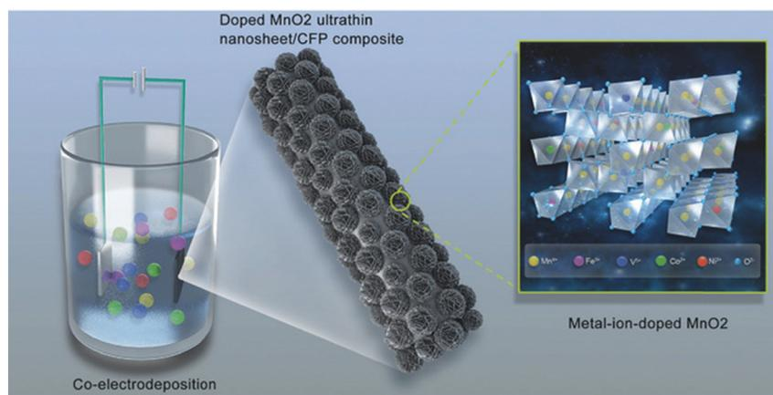
Fig. 24 Schematic representation for the preparation of the metal-ion (Fe, V, Co, Ni)-doped MnO<sub>2</sub> ultrathin nanosheet/CFP composite. Reproduced with permission from ref. 510, Copyright Wiley 2017.
