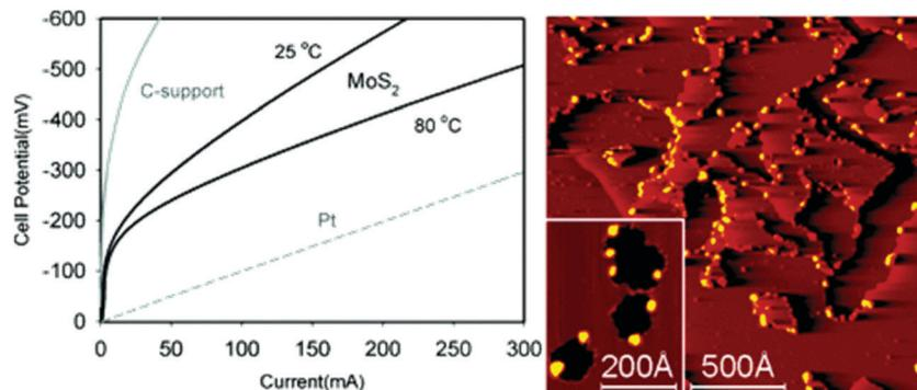
Fig. 76 Polarisation curve for hydrogen evolution on Pt, daihope C-support, and MoS<sub>2</sub> cathodes. The potentials are measured with respect to a carbon-supported Pt anode in a proton exchange membrane electrode assembly. (Right) STM images of MoS<sub>2</sub> nanoparticles on modified graphite. Reproduced with permission from ref. 1137 Copyright 2005 American Chemical Society.
