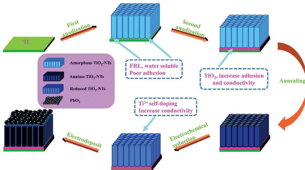
Fig. 21 Schematic representation of the generation of Ti/TiO<sub>2</sub>-NTs/PbO<sub>2</sub>. Reproduced with permission from ref. 488. Copyright Royal Society of Chemistry 2021.
