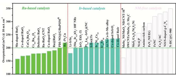
Fig. 20 Comparison of OER overpotentials at 10 mA cm<sup>-2</sup> for the ten most promising catalysts in each category (Ir-, Ru- and PGM-free based catalysts) in acidic media. (a: the overpotential @ 20 mA cm<sup>-2</sup>). Reproduced with permission from ref. 419. Copyright Elsevier 2020
