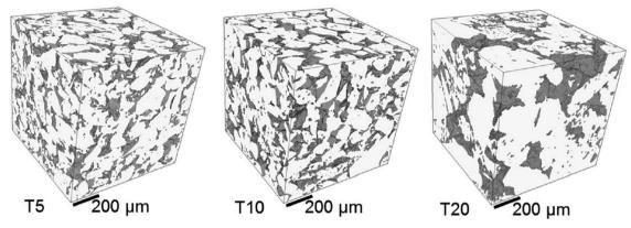
Fig. 146 Example of tomographic elucidation of a PTL porous structure. Reproduced with permission from ref. 1801. Copyright Elsevier 2017.
