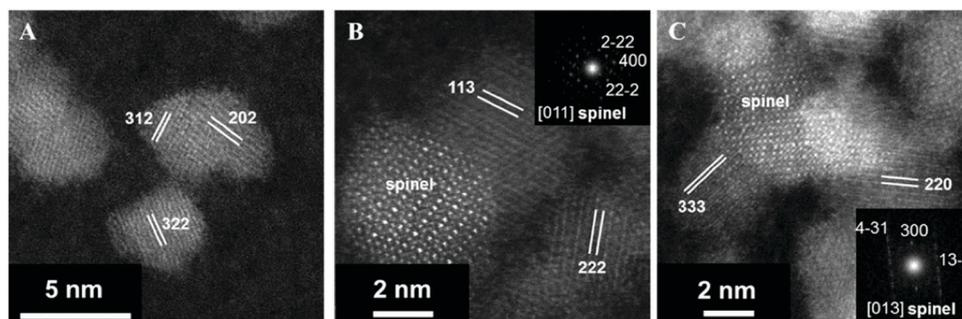
Fig. 39 High-resolution images of spinel-type  $\text{CoV}_{2-x}\text{Fe}_x\text{O}_4$  ( $x = 0–2$ ) nanoparticles: (A)  $\text{CoFe}_2\text{O}_4$ , (B)  $\text{CoFeVO}_4$ , and (C)  $\text{CoV}_2\text{O}_4$ . Reproduced with permission from ref. 703. Copyright American Chemical Society 2018.
