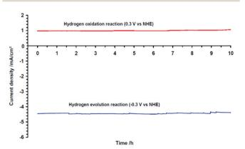
Fig. 137 Long-run electrolysis experiments for both hydrogen evolution and oxidation carried out respectively at -0.3 and +0.3 V vs. NHE in  $H_2SO_4$ (0.5 mol L<sup>-1</sup>) on a membrane electrode on which MWCNTs have been deposited and further Ni-functionalised. Reprinted with permission from ref. 1677 Copyright 2009 AAAS.
