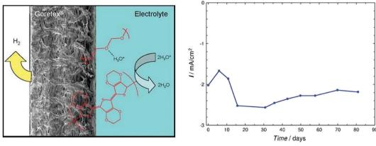
Fig. 94 Schematic of PEDOT-based HER electrode (left side). Long-term performance of PEDOT-PEG on Goretex/Au in 1 M H<sub>2</sub>SO<sub>4</sub> under N<sub>2</sub> at -0.35 V vs. SCE. Reproduced with permission from ref. 1339. Copyright 2010 Wiley.
