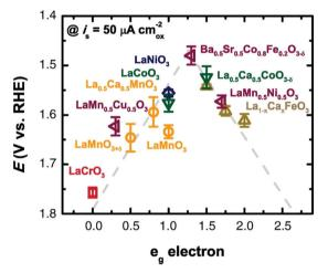
Fig. 30 Relation between observed OER activities of perovskites (ABO $_3$ ) and the number of e $_g$  symmetry electrons of the transition metal (B in ABO $_3$ ). Reproduced with permission from ref. 611. Copyright AAAS 2011.
