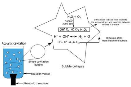
Fig. 147 Production of sonolysis species by acoustic cavitation. 1846
