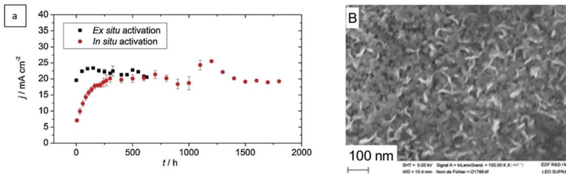
Fig. 112 Comparison of the 316L SS electrodes OER (test conducted at  $E = +1.75$  V vs. RHE) after accelerated activation and the *in situ* activated 316L SS electrodes OER in 5.0 M LiOH at  $T = 25$  °C (A). SEM of the surface of the 316L SS electrode activated (B). Reproduced with permission from ref. 1454. Copyright Elsevier 2019.
