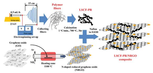
Fig. 33 Schematic presentation of the preparation route leading to perovkite-grapheneoxid composite with special morphology. Reproduced with permission from ref. 667. Copyright Elsevier 2014.
