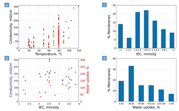
Fig. 10 (a) AEM hydroxide conductivity vs. temperature, and (b) hydroxide conductivity and water uptake of selected AEMs (with conductivities ≥150 mS cm<sup>-1</sup>). (c) Fraction of AEMs at different levels of (c) IEC range and (d) water uptake range. Water uptake values are given in different temperatures. Represented data and the underlying sources are given in Table S1 (ESI†).
