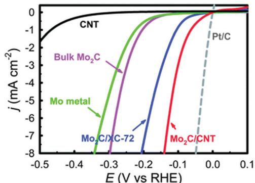
Fig. 60 The polarisation curves of nanostructured  $\text{Mo}_2\text{C}/\text{CNT}$ ,  $\text{Mo}_2\text{C}/\text{XC}$ , bulk  $\text{Mo}_2\text{C}$ , Mo metal, Pt/C and CNT in 0.1 M  $\text{HClO}_4$ . Reproduced with permission from ref. 1348. Copyright RSC 2013.
