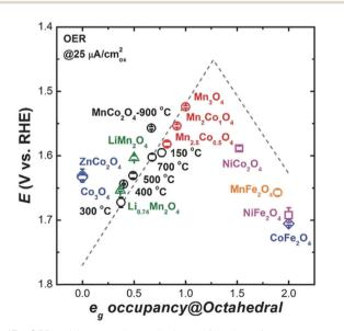
Fig. 43 OER activity on various spinels as a function of e<sub>a</sub> occupancy of the active element at octahedral site. Reproduced with permission from ref. 704. Copyright Wiley 2017.
