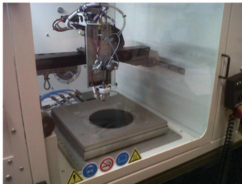
Fig. 109 Photograph of a catalytic ink printer used to spray catalytic inks onto PFSA membranes (batch process, lab-scale). Reproduced with permission from Paris-Saclay University.
