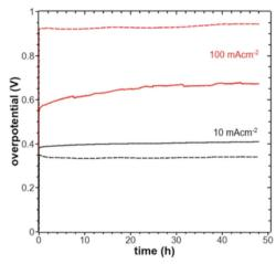
Fig. 38 Plot of the overpotential as a function of time at current densities of 10 mA  $\rm cm^{-2}$  (black) and 100 mA  $\rm cm^{-2}$  (red) measured in 1 M KOH for films deposited at 50  $^{\circ}\text{C}$  (dashed lines) and 103  $^{\circ}\text{C}$  (full lines). Reproduced with permission from ref. 733. Copyright American Chemical Society 2020.
