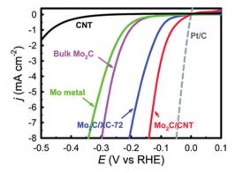
Fig. 60 The polarisation curves of nanostructured Mo<sub>2</sub>C/CNT, Mo<sub>2</sub>C/XC, bulk Mo<sub>2</sub>C, Mo metal, Pt/C and CNT in 0.1 M HClO<sub>4</sub>. Reproduced with permission from ref. 1348. Copyright RSC 2013.
