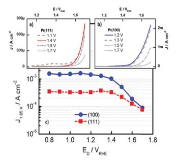
**Fig. 19** LSV curves of (a) Pt(111), (b) Pt(100) in 0.1 M HClO<sub>4</sub> with scan rate of 50 mV s<sup>-1</sup>. (c) Plot of the current density at +1.65 V vs. RHE ( $j_{+1.65V}$ ) in the LSV as a function of the applied potential. Reproduced with permission from ref. 427. Copyright Wiley 2019.
