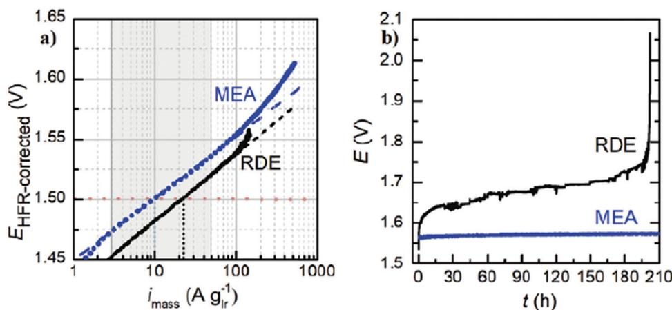
Fig. 144 Evaluation of the OER (a) activity and (b) stability versus time at a given representative OER current in MEA (blue) and RDE (black) configuration for a state-of-the-art commercial  $\text{IrO}_2$  catalyst. Reproduced from ref. 20 with permission from Wiley.
