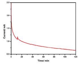
Fig. 132 The charge vs. time and current vs. time plots obtained from chronoamperometric measurements at an applied potential of 1.5 V for two hours to the Co(tpfc)Py<sub>2</sub> -loaded Nafion film. Reprinted with permission from ref. 1577 Copyright 2020 American Chemical Society.
