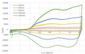
Fig. 101 (left) SEM micrographs of unsupported IrO2 nanoparticles used at the anode of PEM water electrolysis cells. (right) In situ cyclic voltammograms recorded on IrO2 at the anode of a PEM water electrolysis cell, at different scan rates. Reproduced with permission from ref. 116. Copyright Elsevier 2016.
