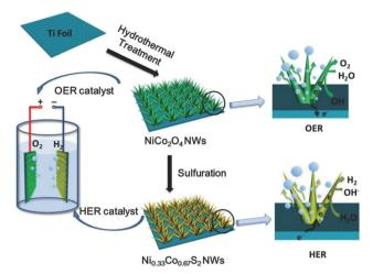
Fig. 45 Schematic illustration of the synthesis of NiCo<sub>2</sub>O<sub>4</sub> and Ni<sub>0.33</sub>Co<sub>0.67</sub>S<sub>2</sub> nanowires, and the utilisation of these homologous Ni-Co based nanowires as OER and HER catalysts for water splitting. Reproduced with permission from ref. 796. Copyright Wiley 2015.
