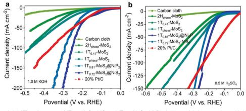
Fig. 83 The electrocatalytic HER performance of  $1T_{0.72}$ -MoS<sub>2</sub>@NiS<sub>2</sub> and  $1T_{0.81}$ -MoS<sub>2</sub>@Ni<sub>2</sub>P hybrid materials in comparison with MoS<sub>2</sub>, carbon cloth and Pt/C. (a) LSV curves in 1 M KOH. (b) LSV curves in 0.5 M H<sub>2</sub>SO<sub>4</sub>. Reproduced with permission from ref. 1185 Copyright Nature Publishing 2021.
