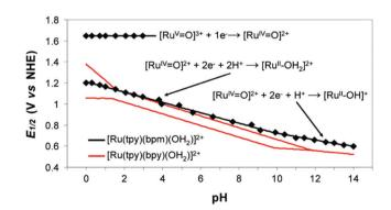
**Fig. 120** Plots of *E*1/2 (V vs. NHE) vs. pH for the Ru(v/iv) and Ru(iv/ii) redox couples of [Ru(tpy)(bpm)(OH<sub>2</sub>)]<sup>2+</sup> and for the Ru(iv/iii) and Ru(iii/ii) redox couples of [Ru(tpy)(bpy)(OH<sub>2</sub>)]<sup>2+</sup> in aqueous solution (I) 0.1 M; T) 298 K; glassy carbon working electrode). Reprinted with permission from ref. 1479 Copyright 2008. American Chemical Society.
