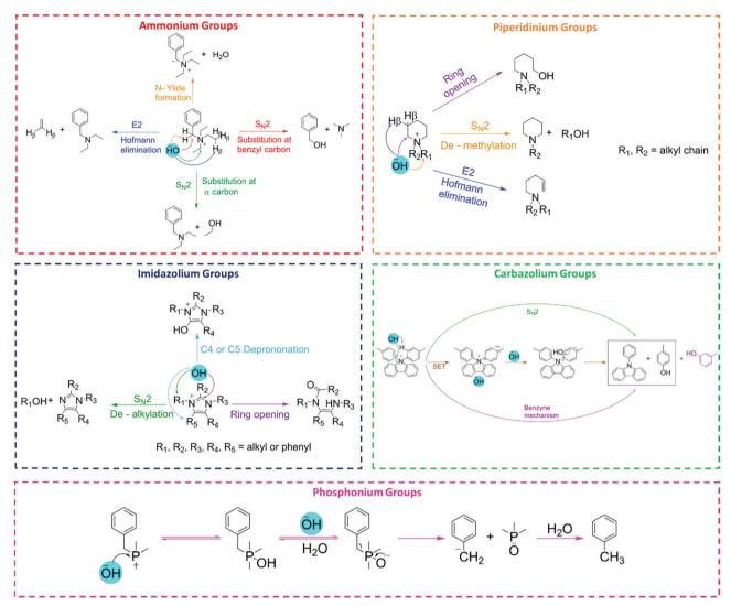
Different degradation mechanisms reported for cationic functional groups in AEMs
