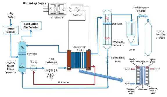
Typcial schematic of a PEMWE system. Source ref. 1908:
