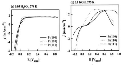
Fig. 18 Polarisation curves for hydrogen evolution/oxidation on Pt(hkl), with scan rate of 20 mV s<sup>-1</sup>, in (a) acid and (b) alkaline media. Reproduced with permission from ref. 409 (copyright MDPI 2020), 410 (copyright American Chemical Society 1997), 412 (copyright RSC 1996).
