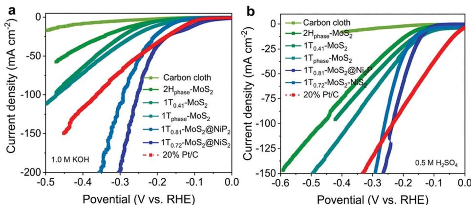
Fig. 83 The electrocatalytic HER performance of  $1T_{0.72}$ - $\text{MoS}_2$ @ $\text{NiS}_2$  and  $1T_{0.81}$ - $\text{MoS}_2$ @ $\text{Ni}_2\text{P}$  hybrid materials in comparison with  $\text{MoS}_2$ , carbon cloth and Pt/C. (a) LSV curves in 1 M KOH. (b) LSV curves in 0.5 M  $\text{H}_2\text{SO}_4$ . Reproduced with permission from ref. 1185 Copyright Nature Publishing 2021.
