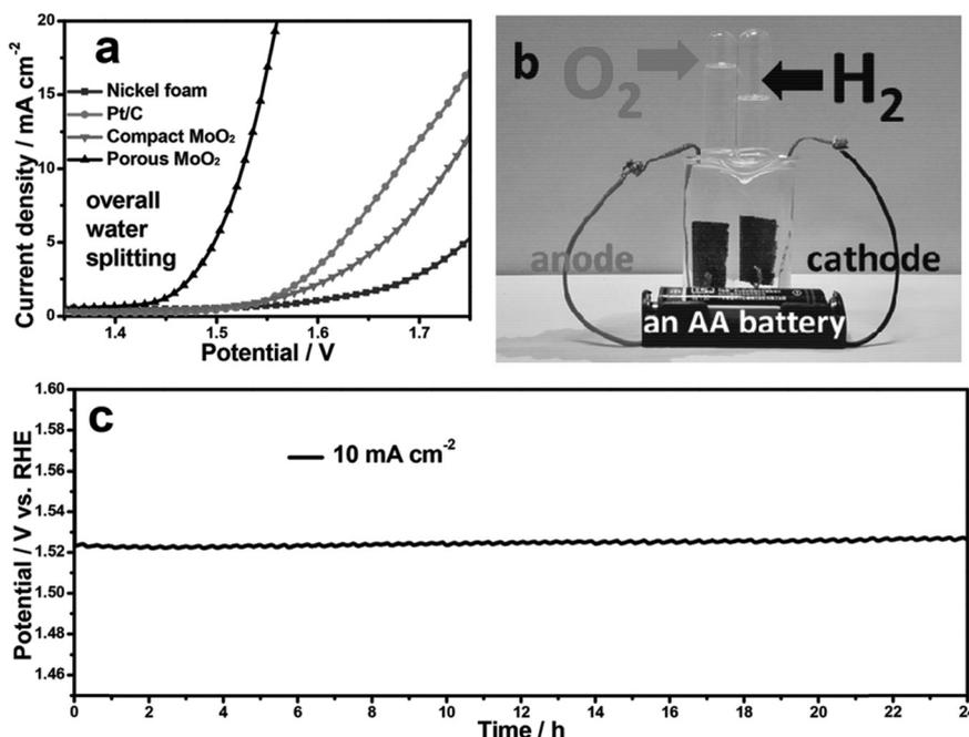
Fig. 26 Steady-state polarisation curves for overall water splitting of Ni foam, commercial Pt/C, compact MoO<sub>2</sub>, and porous MoO<sub>2</sub> in a two-electrode configuration. (b) Demonstration of water-splitting device. (c) Chronopotentiometric curve of water electrolysis for porous MoO<sub>2</sub>. Reproduced with permission from ref. 529 Copyright Wiley 2016.
