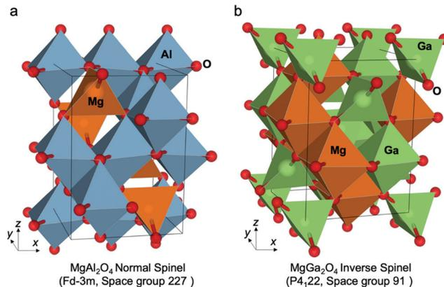
Fig. 36 Normal and inverse spinel structures. (a)  $\text{MgAl}_2\text{O}_4$  normal and (b)  $\text{MgGa}_2\text{O}_4$  inverse ground state atomic configurations. In each case the unit cell is shown by solid black lines. Octahedral and tetrahedral atomic coordination environments are also identified by the coordination polyhedra in each case. Reproduced with permission from ref. 717. Copyright Nature Publishing 2020.
