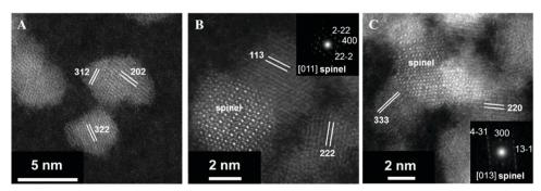
Fig. 39 High-resolution images of spinel-type  $CoV_{2-x}Fe_xO_4$  (x = 0-2) nanoparticles: (A)  $CoFe_2O_4$ , (B)  $CoFe_2O_4$ , and (C)  $CoV_2O_4$ . Reproduced with permission from ref. 703. Copyright American Chemical Society 2018.
