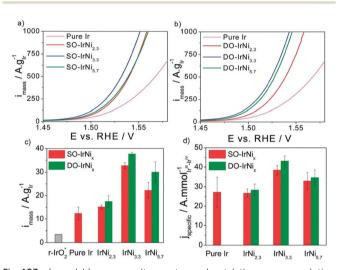
Fig. 103 (a and b) sweep voltammetry and catalytic oxygen evolution reaction (OER) activities of stepwise oxidised (SO) IrNix and directly oxidised (DO) IrNi, core-shell nanoparticles, compared to pure Ir nanoparticles. (c) Ir mass-based activities and (d) specific activities at 0.25 V overpotential. Reproduced with permission from ref. 1429. Copyright RSC 2014
