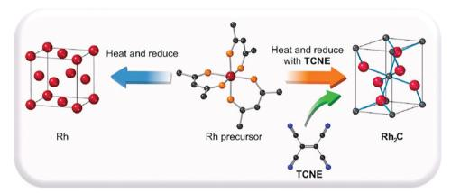
Fig. 64 Schematic presentation of the synthesis of Rh<sub>2</sub>C. Reproduced with permission from ref. 1003. Copyright American Chemical Society 2020.
