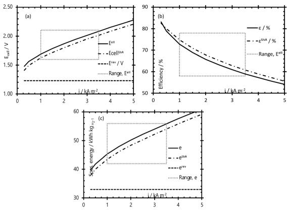
Fig. 148 Effect of ultrasound on (a) cell voltage ( $E_{cell}$ ), (b) efficiency ( $\epsilon$ ) and (c) specific energy (e) for hydrogen production (\*UsA = ultrasoundassisted). 1841
