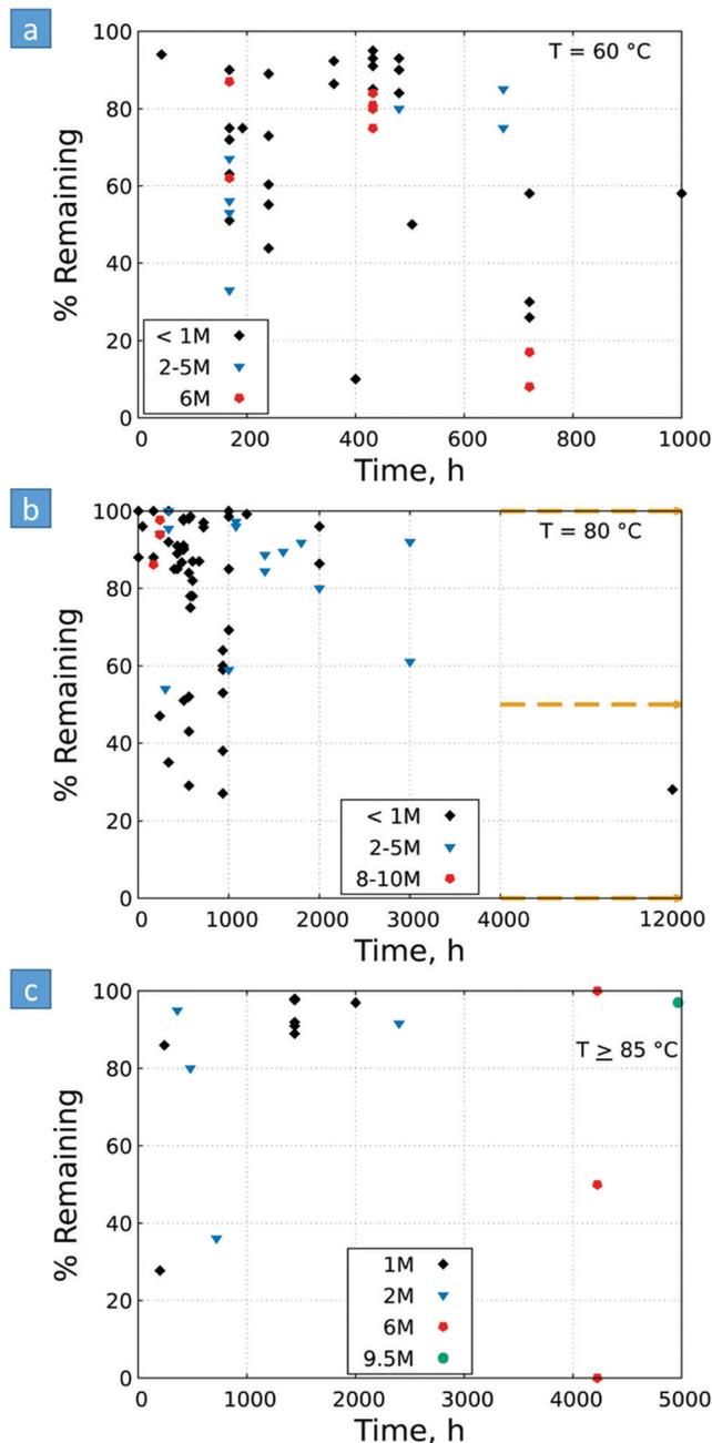
Fig. 16 *Ex situ* alkaline stability data of AEMs. The stability is reported as % QA cation remaining vs. time of stability test, performed in various base concentrations at constant temperatures of (a) 60 °C, (b) 80 °C, and (c)  $\geq 85$  °C. Represented data and underlying sources are given in Table S2 (ESI $\dagger$ ).
