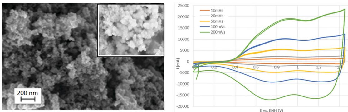
Fig. 101 (left) SEM micrographs of unsupported IrO<sub>2</sub> nanoparticles used at the anode of PEM water electrolysis cells. (right) *In situ* cyclic voltammograms recorded on IrO<sub>2</sub> at the anode of a PEM water electrolysis cell, at different scan rates. Reproduced with permission from ref. 116. Copyright Elsevier 2016.
