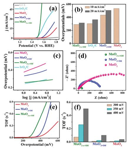
Fig. 27 Polarisation curves toward the OER for as-grown  $MoO_{2+OH^-}$  (7 h case),  $MoO_{2-x+OH^-}$  (9 h case), commercially available  $MoO_2$ , and  $IrO_2/C$ electrocatalysts on GCE in 1 M KOH electrolyte. Reproduced with permission from ref. 531. Copyright American Chemical Society 2020
