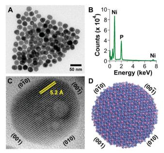
Fig. 71 (A) TEM image and (B) EDX spectrum of Ni<sub>2</sub>P nanoparticles. (C) HRTEM image of a representative Ni<sub>2</sub>P nanoparticle, highlighting the exposed Ni<sub>2</sub>P(001) facet and the 5.2 Å lattice fringes that correspond to the (010) planes. (D) Proposed structural model of the Ni<sub>2</sub>P nanoparticles. Reproduced with permission from ref. 1259 Copyright 2013 American Chemical Society
