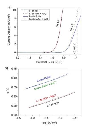
Fig. 151 (a) Electrocatalytic OER activities of NiFe LDH nanoplates supported on carbon, measured using LSV in four different electrolytes after CV "break-in" (50 cycles). A potential of approximately 480 mV, corresponding to the design criteria limit, is marked by a dashed vertical line. (b) Corresponding Tafel plot for low current density j. Measurement conditions: room temperature, 1600 rpm, and scan rate of 1 mV s $^{-1}$ . Reproduced with permission from ref. 1864. Copyright Wiley 2016.
