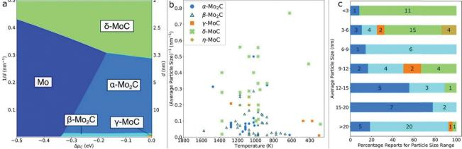
Fig. 66 (a) Lowest energy 2-D phase diagram by projecting 3-D diagram onto  $\Delta\mu_C - 1/d$  axis. (b) Inverse average particle size vs. temperature for experimental reports. For clarity, plasma-based syntheses were omitted from Fig. 66b. (c) Stacked bar graph for percentage of experimental reports at given average particle sizes. Reproduced with permission from ref. 1005. Copyright American Chemical Society 2020.
