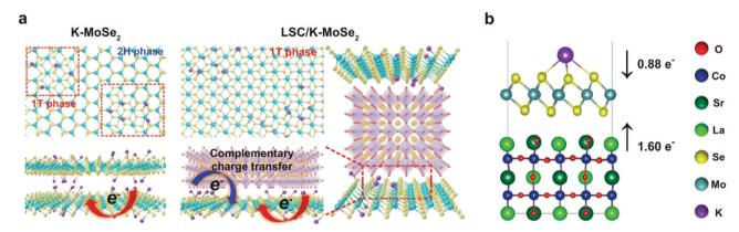
Fig. 34 (a) Schematic of the atomic structure and charge transfer effect for K-MoSe<sub>2</sub> and LSC/K-MoSe<sub>2</sub>. Complementary charge transfer in LSC/K-MoSe<sub>2</sub> can modulate the electronic structure of MoSe<sub>2</sub>, increasing the 1T-MoSe<sub>2</sub> ratio in the heterostructure. (b) Charge transfer from K and LSC to MoSe<sub>2</sub> in the optimised LSC/K-MoSe<sub>2</sub> heterostructure. Reproduced with permission from ref. 684. Copyright Nature Publishing 2021.
