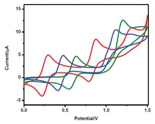
Fig. 131 Water oxidation in the presence of Co(tpc)Py<sub>2</sub> (red), Co(tdfc)Py<sub>2</sub> (blue) and Co(tpfc)Py<sub>2</sub> (green) in acetonitrile on adding 4.8% water. Reprinted with permission from ref. 1577 Copyright 2020. American Chemical Society.
