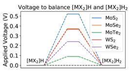
Fig. 77 Required applied potential to obtain a zero-reaction energy for the rate determining Volmer step from [MX<sub>2</sub>]H to [MX<sub>2</sub>]H<sub>2</sub>. Reproduced with permission from ref. 1138 Copyright 2018 American Chemical Society.
