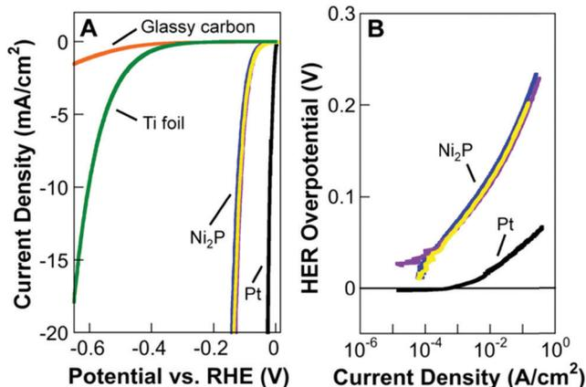
Fig. 72 (A) Polarisation data for three individual  $\text{Ni}_2\text{P}$  electrodes in 0.5 M  $\text{H}_2\text{SO}_4$ , along with glassy carbon, Ti foil, and Pt in 0.5 M  $\text{H}_2\text{SO}_4$ , for comparison. (B) Corresponding Tafel plots for the  $\text{Ni}_2\text{P}$  and Pt electrodes. Reproduced with permission from ref. 1259 Copyright 2013 American Chemical Society.
