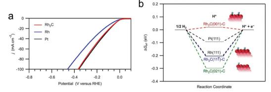
Fig. 65 (a) The HER polarisation curves of 20 wt% Rh<sub>2</sub>C/C (red), Pt/C (black), and Rh/C (blue). The data were recorded in a 1.0 M KOH electrolyte with a scan rate of 50 mV s<sup>-1</sup>. (b) The 3-state free energy diagram for HER. The structural models show the OH\* pre-covered surfaces used for calculations. The blue spheres are hydrogen atoms, and the gray spheres are oxygen atoms. Reproduced with permission from ref. 1003. Copyright American Chemical Society 2020.
