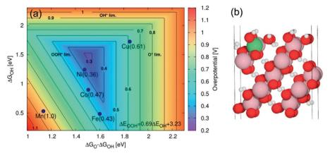
Fig. 42 (a) 2D map of theoretical overpotentials  $\eta$  for the doped  $10\bar{1}4$  surface of  $\beta$ -CoOOH as function of  $\Delta G_{O}-\Delta G_{OH}$  and  $\Delta G_{OH}$ . The individual values of  $\eta$  are indicated in brackets. Improvement in activity relative to undoped surface is obtained in the case of Ni with  $\eta = 0.36$  V and Fe with 0.43 V. Reproduced with permission from ref. 711. Copyright American Chemical Society 2013.
