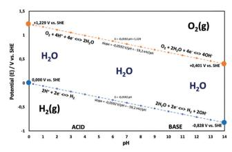
Fig. 2 Water electrolysis electrode potentials with pH at standard conditions. Reproduced with permission from ref. 86. Wiley 2020.
