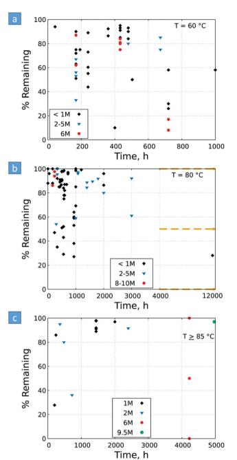
Fig. 16 Ex situ alkaline stability data of AEMs. The stability is reported as % QA cation remaining vs. time of stability test, performed in various base concentrations at constant temperatures of (a) 60 °C, (b) 80 °C, and (c)  $\geq$ 85 °C. Represented data and underlying sources are given in Table S2 (ESI†).
