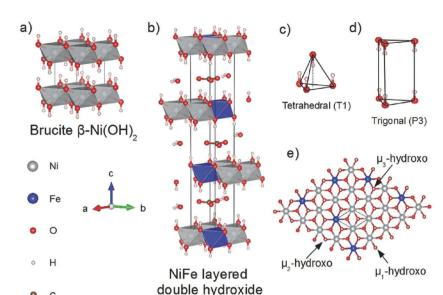
Typical structure of Brucite type Ni(OH)<sub>2</sub> and hydrotalcite-like NiFe LDH. Reproduced with permission from ref. 812. Copyright Wiley 2016.
