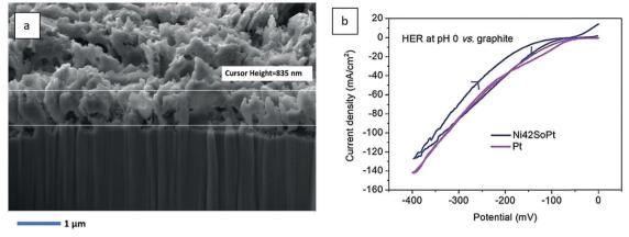
Fig. 106 (a) SEM photograph showing the cross-section of the Ni<sub>42</sub>/Pt interface (Pt thickness ~800-900 nm); the Pt loading is 1.8 mg cm<sup>-2</sup>, (b) comparison of the HER performances of Pt and Ni<sub>42</sub>SoPt at pH = 0. Reproduced with permission from ref. 1269. Copyright Wiley 2019.
