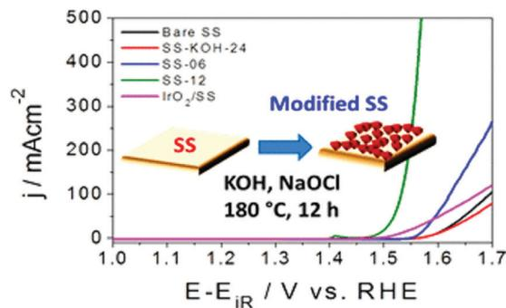
Fig. 87  $\text{Fe}_2\text{O}_3/\text{NiO}$  nanocrystals were formed on the surface of corroded AISI 304 steel and significantly improved the capability of the material to act as an OER electrode. Reproduced with permission from ref. 1285 Copyright American Chemical Society 2017.
