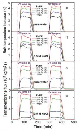
Fig. 17 The effect of Ag NP concentration in PVDF dope solution on (a and b) the bulk feed temperature, and (c and d) water vapor flux in PVMD operated with pure water and 0.5 M NaCl solution. Copyright 2016 Wiley. Used with permission from ref. 278
