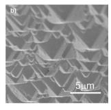
Fig. 11 (a) Schematic illustration of graphdivne/CuO-based multidimensional architecture. Reprinted (adapted) with permission from ref. 247. Copyright 2017 American Chemical Society. (b) The SEM images of the inverted pyramids of the photothermal membrane. Adapted from ref. 248 by permission of The Royal Society of Chemistry.
