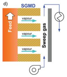
Fig. 1 The four basic membrane distillation configurations: (a) direct contact membrane distillation (DCMD); (b) air gap membrane distillation (AGMD); (c) vacuum membrane distillation (VMD) and, (d) sweep gas membrane distillation (SGMD).
