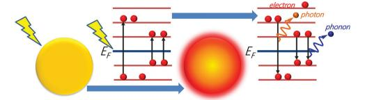
Fig. 4 Decay channels for plasmonic excitation: electron-to-photon, electron-to-electron, and electron-to-phonon
