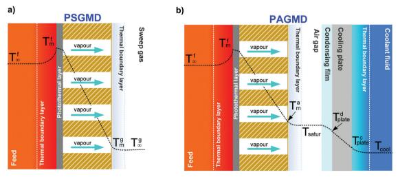
Fig. 16 Temperature profile in: (a) PSGMD and (b) PAGMS configurations.
