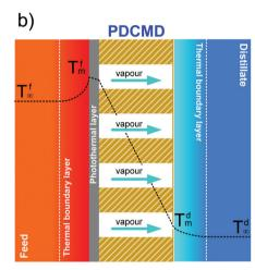
Fig. 2 (a) Temperature profile in the direct contact membrane distillation (DCMD) configuration; (b) photothermal direct contact membrane distillation (PDCMD): the effect of a self-heating membrane surface incorporating metal NPs as localized "nano-heaters" on the temperature profile.
