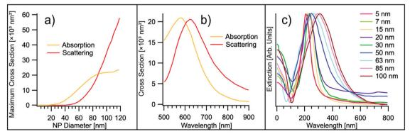
Fig. 5 (a) Evolution of the maximum absorption and scattering cross-section as a function of the NP diameter d for the case-study example of gold. Experimental points are taken from ref. 132. (b) Absorption and scattering cross-section for a gold nanosphere in water, with d = 88 nm. Experimental points are taken from ref. 132. (c) UV-Vis extinction spectra of Ag NPs of different diameters. Experimental points are taken from ref. 142.
