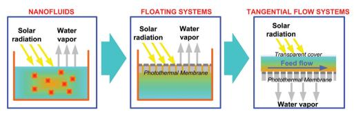
Fig. 9 The evolutionary pathway of photothermal evaporation.
