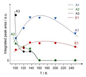
Fig. 7 Integrated peak areas of the vibrational bands of the aldehyde species A1-A3 ( $\nu$ (C=O)) and the enol species E1 ( $\nu$ (C-O)) plotted as a function of surface temperature. The areas were integrated within the rectangles shown in Fig. 6.
