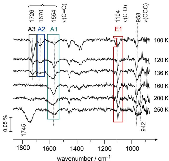
**Fig. 6** Comparison of the IR spectra of butanal adsorbed on Pd(111) obtained at different surface temperatures indicated next to the spectra (100–250 K). The exposure of butanal in all spectra amounts to  $7.8 \times 10^{14} \text{ mol cm}^{-2}$ ; the butanal was dosed at a flux of  $3.7 \times 10^{12} \text{ mol cm}^{-2} \text{ s}^{-1}$ .
