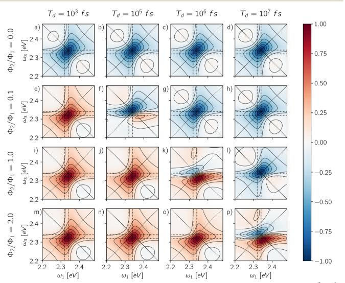
Fig. 6 Rephasing maps for different values of GQY ratio ( $\Phi_2/\Phi_1 = 0.0$ , 0.1, 1.0, 2.0) on the columns and different detection-times ( $T_d = 10^3$  fs,  $10^5$  fs,  $10^6$  fs,  $10^7$  fs) on the rows. Each map is normalized with respect to its absolute maximum/minimum.
