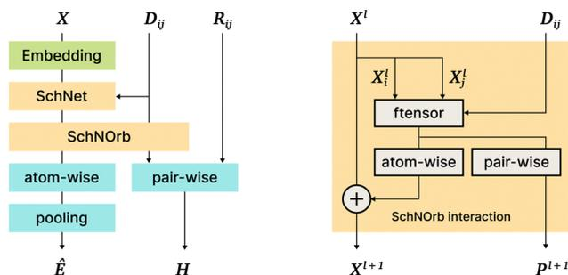
Fig. 6 The *SchNorb* architecture. On the left: general architecture overview; on the right: the Interaction block in *SchNorb*. In addition to the *SchNet* Interaction block, *SchNorb* uses the factorized tensor layer<sup>74</sup> to produce pairwise atom features and predict the basis coefficients for the Hamiltonian.
