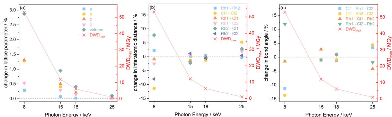
Fig. 7 Structural changes observed in  $[\text{Rh}(\text{COD})\text{Cl}]_2$  at the four photon energies  $h\nu$  (8, 15, 18 and 25 keV) with respect to the maximum diffraction-weighted dose ( $\text{DWD}_{\text{max}}$ ) after 41.7 min of X-ray exposure, including the percentage changes in (a) the lattice parameters  $a$ ,  $b$  and  $c$ , (b) the interatomic distances, and (c) the bond angles.
