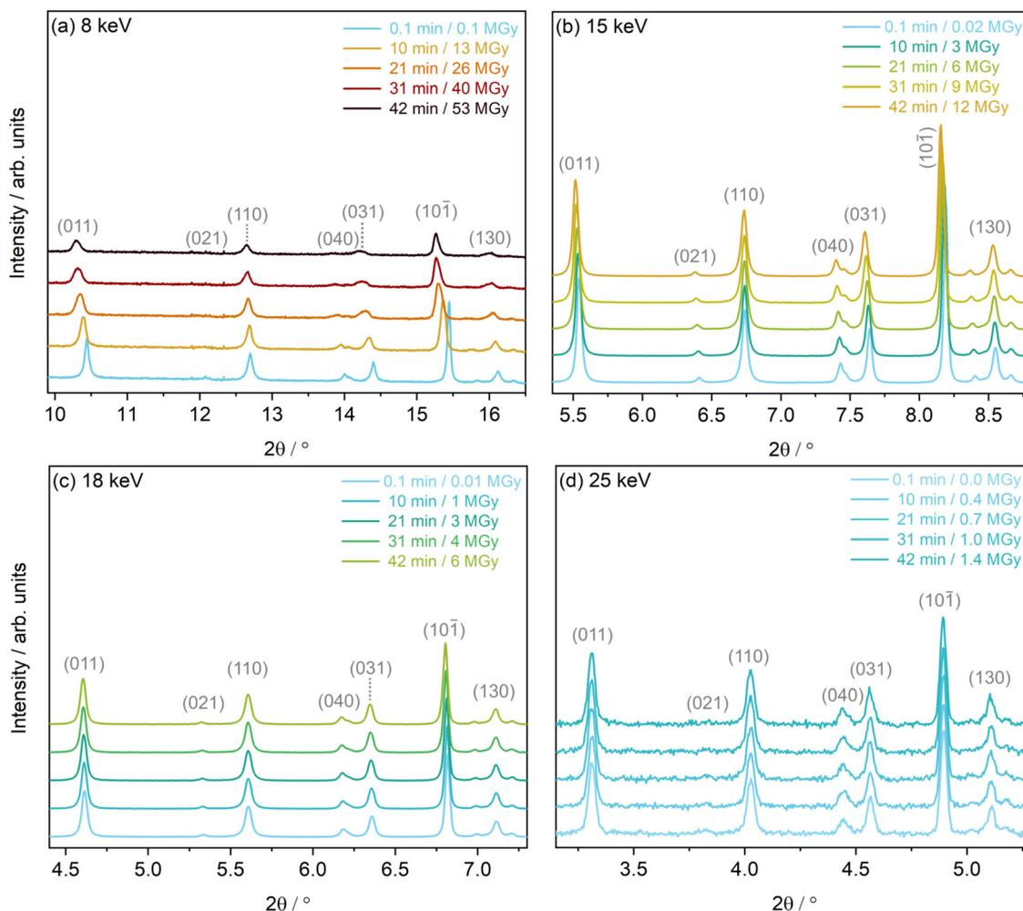
Fig. 4 Discrete powder diffraction patterns of  $[\text{Rh}(\text{COD})\text{Cl}]_2$  of select low angle Bragg peaks collected approximately every 10 min at experimental settings corresponding to photon energies of (a) 8 keV, (b) 15 keV, (c) 18 keV and (d) 25 keV.
