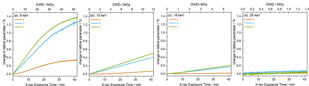
Fig. 5 Change in the lattice parameters *a*, *b* and *c* of [Rh(COD)Cl]<sub>2</sub> as a function of diffraction-weighted dose (DWD) and X-ray exposure time at photon energy setups of (a) 8 keV, (b) 15 keV, (c) 18 keV, and (d) 25 keV.
