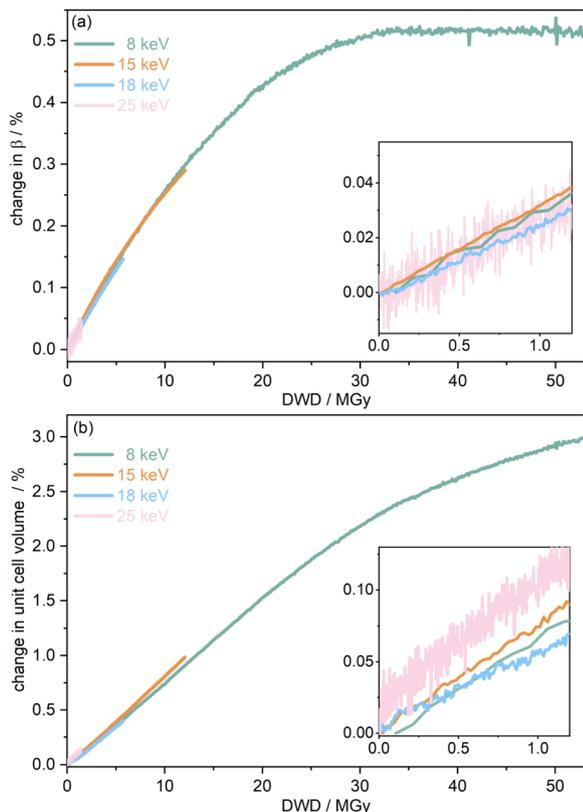
Fig. 6 The percentage change in (a) angle  $\beta$  and (b) unit cell volume  $V$  as a function of diffraction-weighted dose (DWD) at photon energies  $h\nu$  of 8, 15, 18, and 25 keV. The insets show the low dose range up to 1.2 MGy. Note the wide range (order of magnitude difference) in the maximum DWD at the various incident energies.
