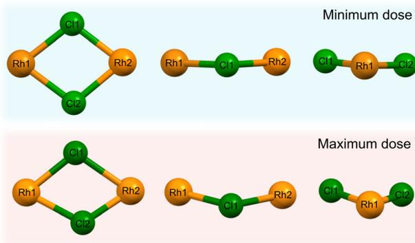
Fig. 8 The central Rh–Cl motif of  $[\text{Rh}(\text{COD})\text{Cl}]_2$  obtained from refinement of the dataset collected at 8 keV photon energy, looking at the Rh–Cl plane and the side profiles, depicting the change in the structure's atomic arrangement as a result of X-ray irradiation. The top row is the minimum dose structure (0.1 MGy,  $t = 5$  s) and the bottom row is the maximum dose (53 MGy,  $t = 41.7$  min) structure.
