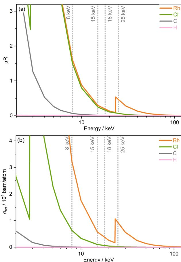
**Fig. 2** Energy-dependence of (a) the absorption coefficients  $\mu R$  obtained from WebAbsorb, Argonne National Laboratory,<sup>47</sup> and (b) the total photoionisation cross sections  $\sigma_{\text{tot}}$  from Scofield for elements present in  $[\text{Rh}(\text{COD})\text{Cl}]_2$ .<sup>48,49</sup>
