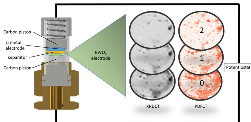
Fig. 1 A sketch of the electrochemical TSCT cell with examples of tomographic slices for the three different axial positions (0, 1, 2) in the  $\text{BiVO}_4$  electrode measured at the start of the *operando* TSCT experiment reconstructed in XRDCT (total diffracted intensity) and PDFCT ( $\text{BiVO}_4$  distribution) modes.
