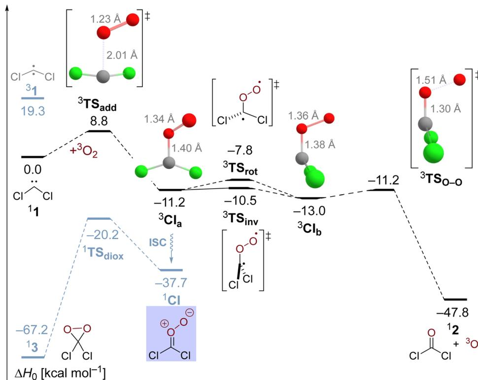
Fig. 1 Potential energy diagram of the dichlorocarbene reaction with molecular oxygen at the estimated BD(TQ)/CBS//CCSD(T)/cc-pVTZ level of theory. The black and blue surfaces correspond to overall triplet and singlet electronic states, respectively.
