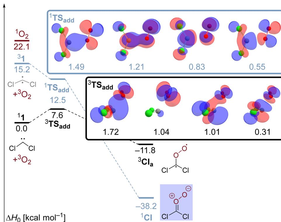
Fig. 2 Potential energy diagram of the dichlorocarbene/ $\text{O}_2$  reaction in overall singlet (blue) and triplet states (black) at the NEVPT2//CASSCF(10e, 8o)/cc-pVTZ level of theory. The insets show selected natural orbitals of the active space and their respective occupation numbers.
