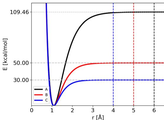
Fig. 1 Morse functions used in the modified CH<sub>4</sub> molecular system: potential A is in black, potential B in red and potential C in blue. Horizontal dotted lines show the corresponding  $D_0$  values, while vertical dashed lines show the position of the threshold distances used in trajectory simulations.
