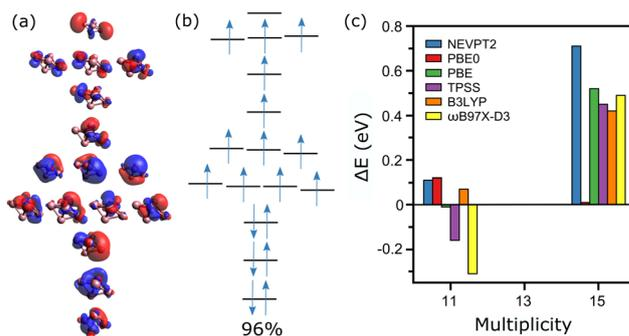
**Fig. 6** (a) Plot of the active orbitals in the CASSCF calculation of  $\text{Co}_5^+$ , ordered in ascending order of energy. (b) Diagram (not to scale) of the electronic levels of  $\text{Co}_5^+$ , with a representation of the electron occupancies in the  $M = 13$  ground-state. (c) Energy differences, with respect to the measured multiplicity state ( $M = 13$ ), for calculations conducted at the NEVPT2, DFT(PBE0), DFT(PBE), DFT(TPSS), DFT(B3LYP) and DFT( $\omega$ B97X-D3) levels of theory.
