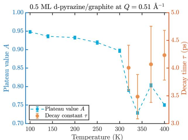
Fig. 8 Temperature dependence of the plateau value  $A$  (blue squares) and the decay time  $\tau$  (orange circles) at a momentum transfer of  $Q = 0.51 \text{ \AA}^{-1}$  from the fitted NSE data according to eqn (2). The strong drop of the static component  $A$  at 320 K confirms the melting temperature determined in the diffraction data while the dynamics occurs within a typical timescale of  $\approx 4 \text{ ps}$ .
