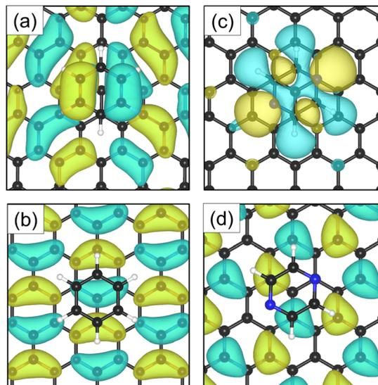
**Fig. 6** Top-view of the HOMO for benzene (a) and pyrazine (c) adsorbed on graphite. The LUMO orbitals are represented in (b) and (d) for benzene and pyrazine, respectively. In the case of  $C_6H_6$ , the  $\pi$  orbitals of the adsorbate and graphite (0001) surface contribute to the HOMO. For  $C_4H_4N_2$ , a larger contribution to the HOMO comes from the adsorbed ring.
