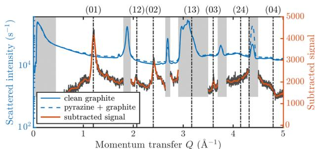
Fig. 2 Diffraction data at 275 K for the pristine graphite sample and a coverage of 0.9 ML of  $C_4D_4N_2$  together with the subtracted data (300 K). Regions with a strong graphite signal are indicated by a grey patch and are omitted in the subsequent analysis.
