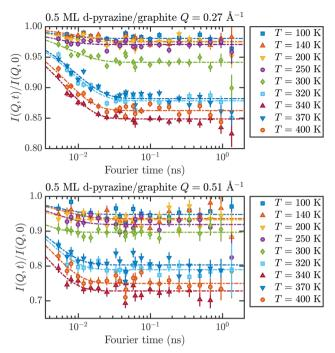
Fig. 7 Neutron spin-echo spectra of a 0.5 ML pyrazine on graphite sample, measured at temperatures between 100 and 400 K at a momentum transfer of  $Q = 0.27 \,\text{Å}^{-1}$  (upper graph) and  $Q = 0.51 \,\text{Å}^{-1}$ . The single spectra have been fitted by exponential decay functions according to eqn (2).
