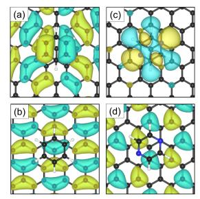
Fig. 6 Top-view of the HOMO for benzene (a) and pyrazine (c) adsorbed on graphite. The LUMO orbitals are represented in (b) and (d) for benzene and pyrazine, respectively. In the case of  $C_6H_{6}$ , the  $\pi$  orbitals of the adsorbate and graphite (0001) surface contribute to the HOMO. For C<sub>4</sub>H<sub>4</sub>N<sub>2</sub>, a larger contribution to the HOMO comes from the adsorbed ring.
