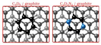
Fig. 1 Graphical impression of the heterocyclic organic molecules benzene  $(C_6D_6)$  and pyrazine  $(C_4D_4N_2)$  adsorbed on graphite.
