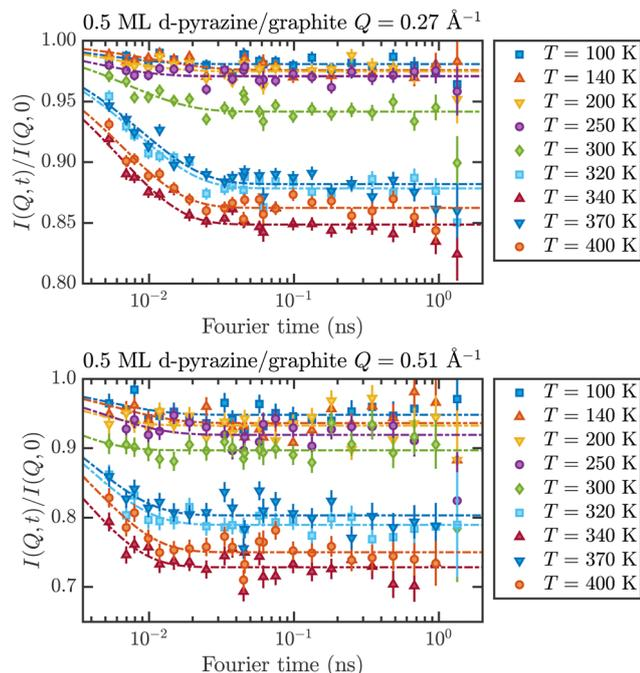
Fig. 7 Neutron spin-echo spectra of a 0.5 ML pyrazine on graphite sample, measured at temperatures between 100 and 400 K at a momentum transfer of  $Q = 0.27 \text{ \AA}^{-1}$  (upper graph) and  $Q = 0.51 \text{ \AA}^{-1}$ . The single spectra have been fitted by exponential decay functions according to eqn (2).
