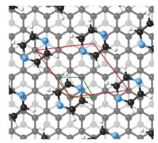
Fig. 4 Proposed structure of a pyrazine (C<sub>4</sub>H<sub>4</sub>N<sub>2</sub>) monolayer adsorbed on graphite. Placement of the experimentally determined periodic pyrazine overlayer on graphite (0001) corresponds to an incommensurate (2.52  $\times$ 2.52)R6.6° superstructure as illustrated by the red dashed rhombus.
