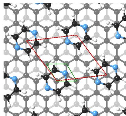
**Fig. 4** Proposed structure of a pyrazine ( $C_4H_4N_2$ ) monolayer adsorbed on graphite. Placement of the experimentally determined periodic pyrazine overlayer on graphite (0001) corresponds to an incommensurate  $(2.52 \times 2.52)R6.6^\circ$  superstructure as illustrated by the red dashed rhombus.
