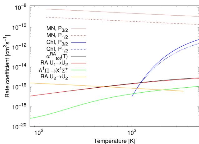
Fig. 3 Rate coefficients for studied processes: for mutual neutralisation (MN), chemiionisation (ChI), and radiative association (RA).  $\alpha_{\text{tot}}^{\text{RA}}$  is a total rate coefficient for formation of NaCl by radiative association of neutral atoms (by summing over processes (1) and (3)). The results for radiative association of the neutral atoms up to 750 K are taken from Šimsová-Zámcniková *et al.*<sup>11</sup>
