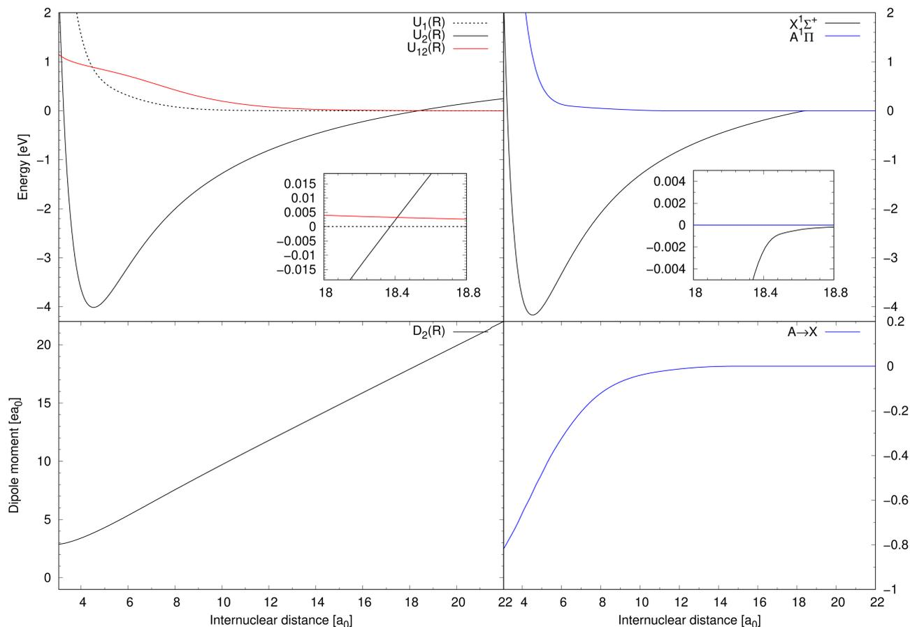
Fig. 1 Top-left: The potential energy curves of two lowest  $1\Sigma^+$  diabatic electronic states of NaCl and the diabatic coupling between them.<sup>20</sup> Bottom-left: The dipole-moment function for the diabatic ionic state.<sup>20</sup> Top-right: The Born–Oppenheimer potential energy curves for the  $A^1\Pi$  and  $X^1\Sigma^+$  states.<sup>20,27</sup> Bottom-right: The transition dipole-moment function for the  $A^1\Pi \rightarrow X^1\Sigma^+$  transitions.<sup>27</sup>
