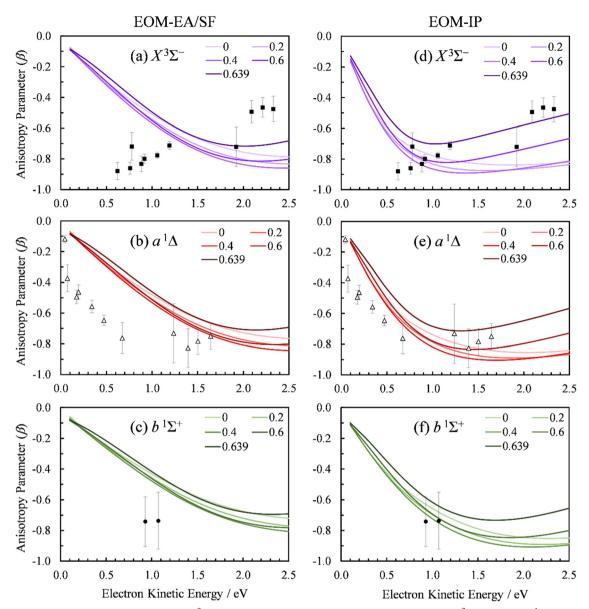
Fig. 10 Experimental and computed PADs for SO $^-$  (X $^2\Pi$ ) photodetachment to the SO neutral states: (a) and (d) X $^3\Sigma^-$ , (b) and (e) a $^1\Delta$ , (c) and (f) b $^1\Sigma^+$ . The calculations in the left column (a)–(c) used the EOM-EA/SF-CCSD Dyson orbitals; those on the right (d)–(f)–EOM-IP-CCSD. PADs calculated with varying point dipole strength (in a.u.) are shown. Symbols represent the experimental data reproduced from Fig. 2(a).
