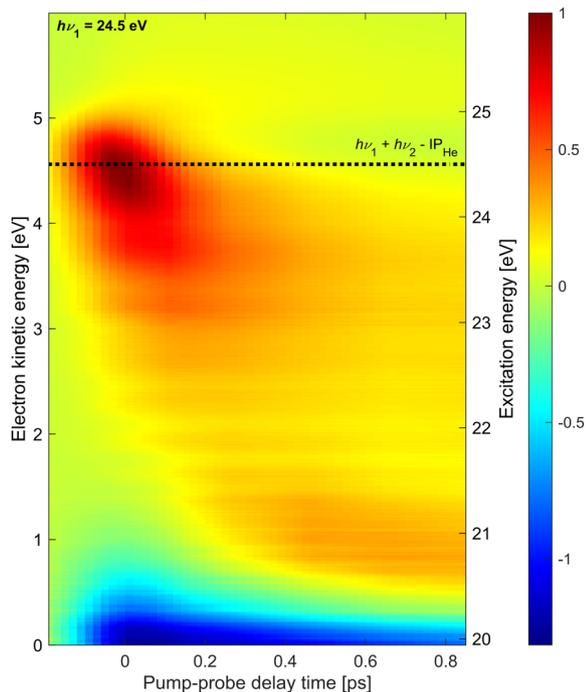
Fig. 4 Time-resolved photoelectron spectra recorded at  $h\nu_1 = 24.5$  eV composed of 13 spectra at different pump–probe delays. The dashed line indicates the expected electron energy for direct  $1 + 1'$  photoionization.
