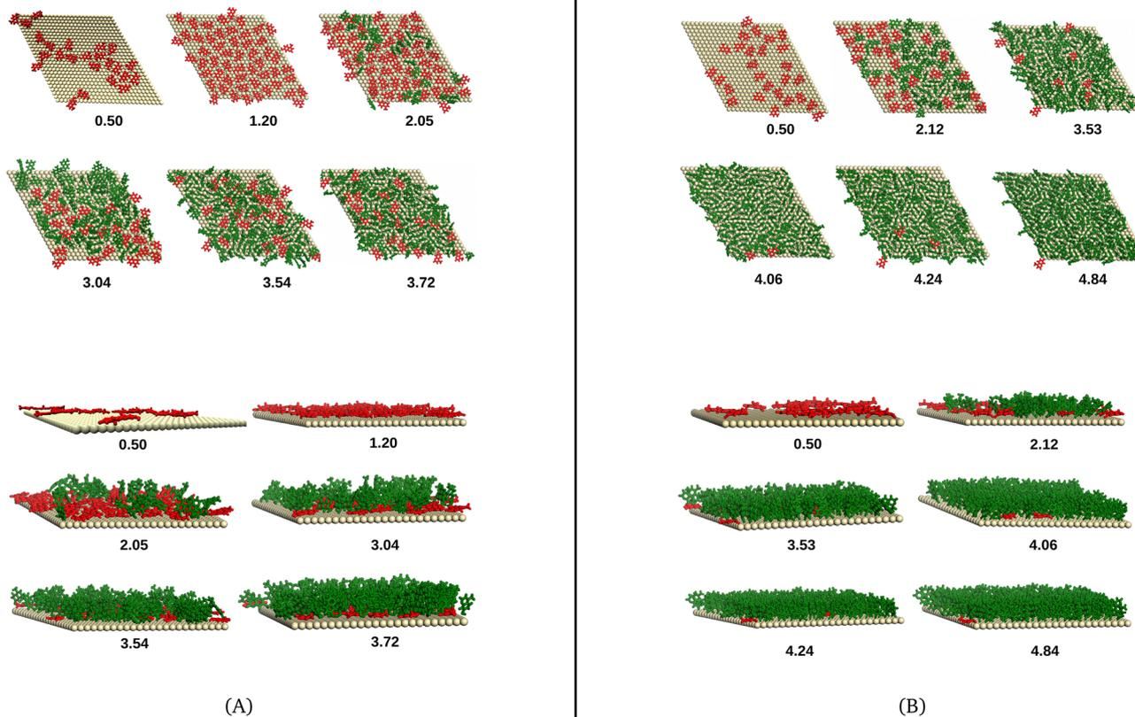
Fig. 2 MD snapshots (top and side views) of: thiol (A) and thiyl (B) SAMs with different number densities ( $\text{nm}^{-2}$ ) (indicated below each image). In red/green molecules in horizontal/vertical arrangement.
