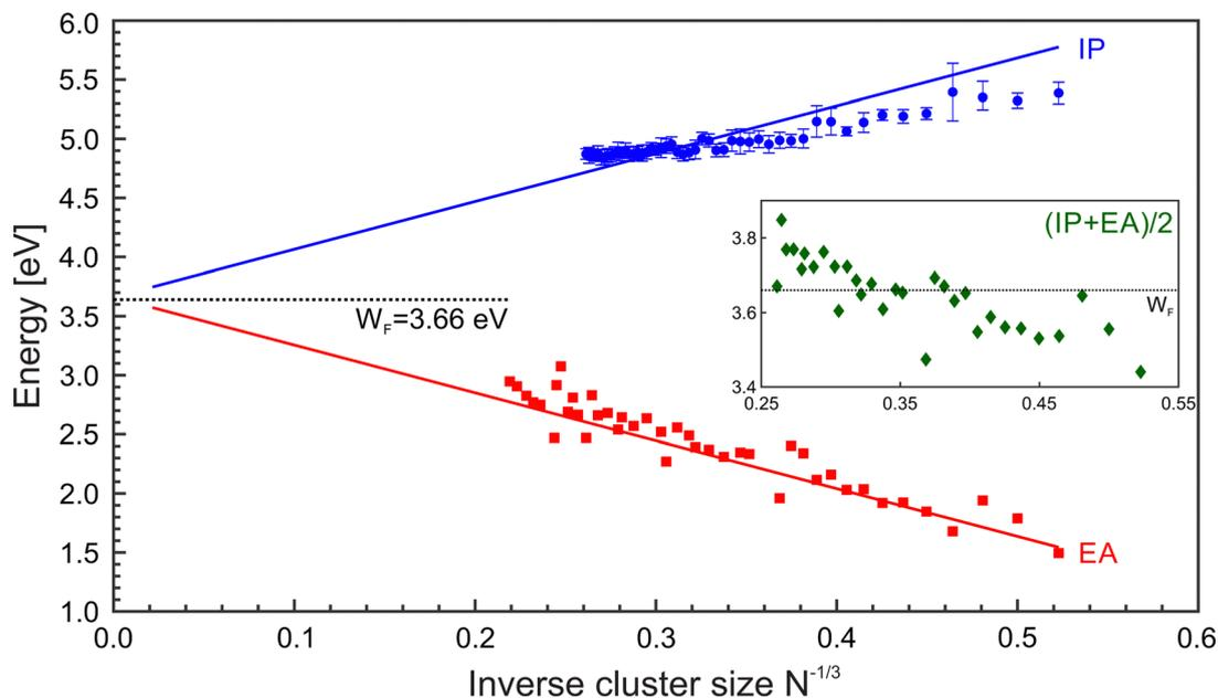
Fig. 6 Ionization potentials (IP, blue  $\circ$ ), electron affinities (EA, black  $\square$ ), and Mulliken electronegativity ( $\chi = (IP + EA)/2$ , green  $\diamond$ ) of  $Mg_N$  as a function of  $N^{-1/3}$ . Lines corresponds to the liquid drop model (LDM) based on eqn (2) and (3) with  $\alpha = \beta = 1/2$ . The black dotted line shows the bulk work function. The EAs have been taken from.<sup>42,48</sup>
