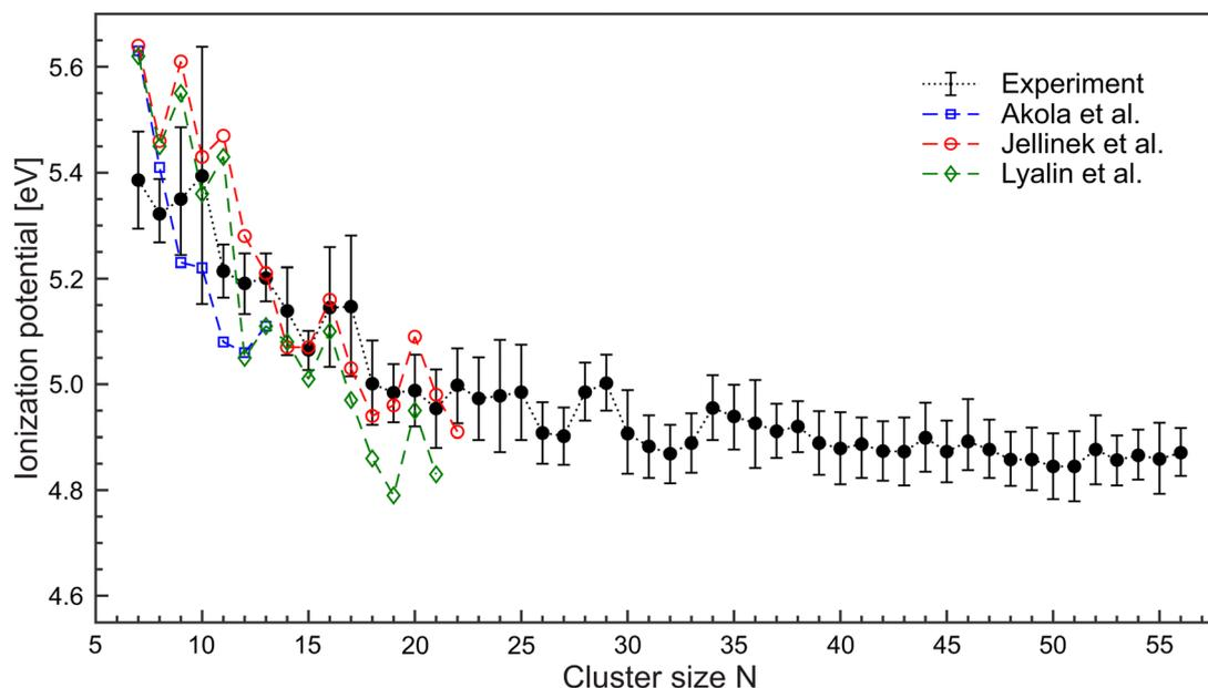
Fig. 4 Ionization potentials of  $Mg_N$  in the size range  $N = 7-56$  (black  $\bullet$ ) extracted from the ionization efficiency curves. DFT-calculations on  $Mg_N$  have been conducted by Akola *et al.*<sup>36</sup> (blue  $\square$ ), Jellinek *et al.*<sup>37</sup> (red  $\circ$ ) and Lyalin *et al.*<sup>38</sup> (green  $\diamond$ ). Lines are used to guide the eyes.
