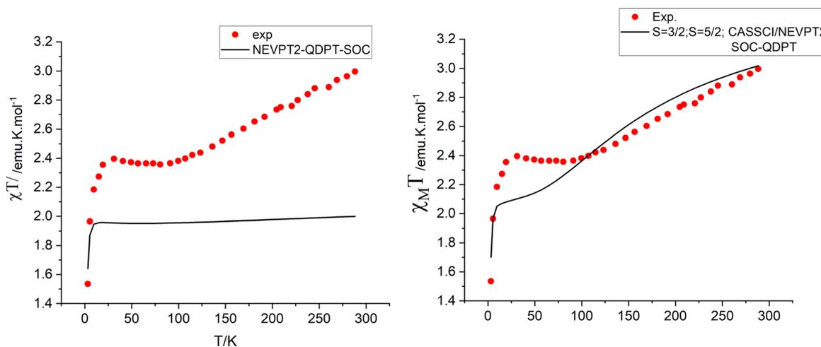
**Fig. 8** Experimental (red points) and simulated  $\chi T$  vs.  $T$  dependencies from spin-orbit coupling calculations using the manifold of 40 lowest  $S = 3/2$  scalar relativistic roots (left) and including in addition the manifold of 40 lowest  $S = 5/2$  roots (right). The latter results explain the increase of  $\chi T$  at  $T > 100$  K with Boltzmann populations of excited  $S = 5/2$  levels (see Table 6).
