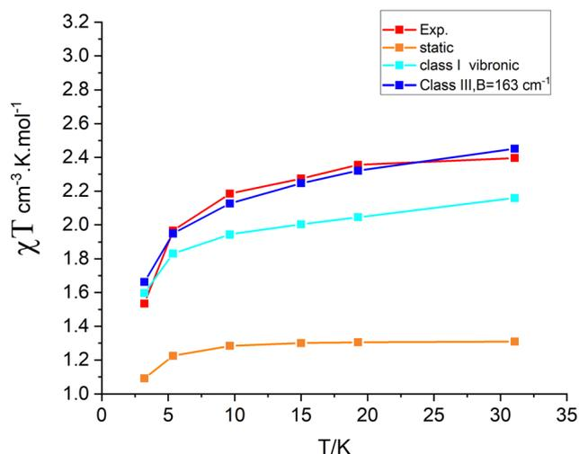
Fig. 13 Comparison between experimental ("Exp") and theoretical  $\chi T$  vs.  $T$  dependencies using the static geometry of  $\mathbf{3}'$  and vibronic wave functions computed using Class I and Class III models.
