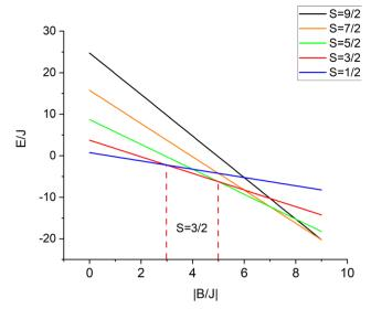
Fig. 3 Energies of spin levels E(S, -)/J versus the |B/J| ratio; in a 3 < |B/J|< 5 range the = 3/2 state is stabilized with respect to the other spin states.
