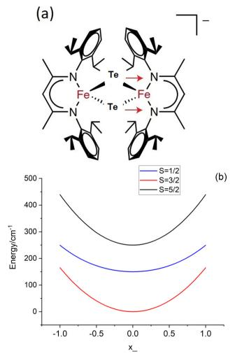
Fig. 4 (a) Representation of the anion  $[L_2Fe_{2\mu}Te_2]^-$ , the red arrows depict the asymmetric (symmetry breaking) mode (q); (b) adiabatic ground state (S = 3/2) and two lowest (S = 1/2, S = 5/2) excited states along q; The curves were plotted taking the values of  $J = -200 \text{ cm}^{-1}$  and  $B = -200 \text{ cm}^{-1}$ 750 cm<sup>-1</sup> (from ref. 10) and the vibronic coupling energy  $\lambda = 480 \text{ cm}^{-1}$ (see Table 7).
