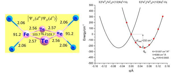
Fig. 9 The centrosymmetric geometry of  $\mathbf{3}'$  (left) used as reference (q = 0) to scan the potential surface along the symmetry breaking local mode q (right).
