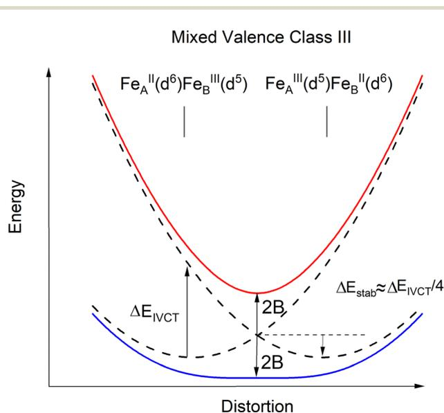
Fig. 11 Configuration energy diagram (schematic) for  $3'$  in the limit of a complete delocalization of the extra electron over the two iron sites ( $\text{Fe}^{2.5+}_{\mu}\text{Te}_2\text{Fe}^{2.5+}$ , Class III).
