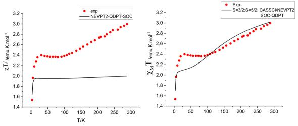
Fig. 8 Experimental (red points) and simulated  $\gamma T$  vs. T dependencies from spin-orbit coupling calculations using the manifold of 40 lowest S=3/2scalar relativistic roots (left) and including in addition the manifold of 40 lowest S = 5/2 roots (right). The latter results explain the increase of  $\chi T$  at T > 5100 K with Boltzmann populations of excited S = 5/2 levels (see Table 6).
