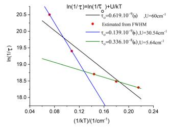
Fig. 14 Spin-relaxation rates from Lorentzian broadening of the low-field sharp line transition in the X-Band EPR spectrum of 3 (red points);<sup>10</sup> simulation of the data using a single exponential Orbach relaxation mechanism (black line), and simulation of the data using a biexponential Orbach mechanism, blue line (T = 20, 13.3 K data points), green line (T = 10, 8, 6.7 K data points).
