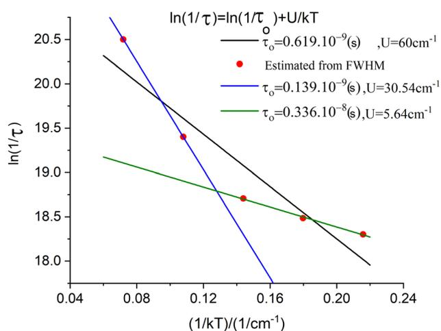
Fig. 14 Spin-relaxation rates from Lorentzian broadening of the low-field sharp line transition in the X-Band EPR spectrum of  $\mathbf{3}$  (red points);<sup>10</sup> simulation of the data using a single exponential Orbach relaxation mechanism (black line), and simulation of the data using a bi-exponential Orbach mechanism, blue line ( $T = 20, 13.3 \text{ K}$  data points), green line ( $T = 10, 8, 6.7 \text{ K}$  data points).
