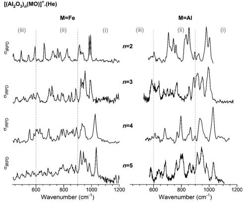
Fig. 1 Experimental IRPD spectra of He-tagged ( $Al_2O_3$ ) $_n$ (MO)<sup>+</sup> with n=2-5. Spectra for M=Fe (present study, singly He-tagged clusters) are shown on the left-hand side and those for M = Al (from ref. 27, multiple He-tagging) on the right-hand side panel. See Table S2, ESI† for band positions and assignments. Three characteristic spectral regions are indicated by the dashed lines: (i) 1200-900, (ii) 900-600, and (iii) < 600 cm<sup>-1</sup>.
