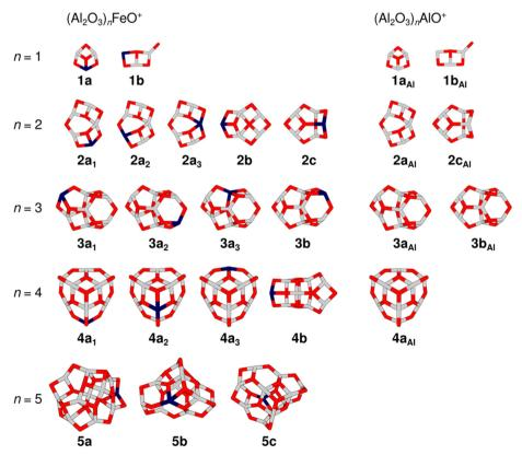
Fig. 2 Overview of TPSSh/def2-TZVP low-energy isomers of (Al<sub>2</sub>O<sub>3</sub>)<sub>n</sub>FeO<sup>+</sup> (left-hand side) and (Al<sub>2</sub>O<sub>3</sub>)<sub>n</sub>AlO<sup>+</sup> (right-hand side). Isomer labels are given below each structure (gray: aluminium, dark blue: iron, red: oxygen). Table S1 in the ESI† lists the relative energies of the isomers.
