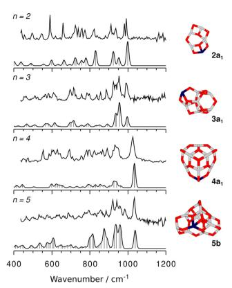
Fig. 3 Experimental IRPD spectra of He-tagged  $(Al_2O_3)_nFeO^+$  (upper trace in each panel) compared with the scaled harmonic TPSSh/def2-TZVP spectra (lower trace in each panel, scaling factor: 1.0175) of the (untagged) assigned isomers. On the right-hand side the respective isomers are depicted (gray: aluminium, dark blue: iron, red: oxygen).
