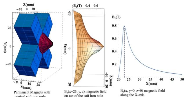
Fig. 1 The magnetic field configuration calculated by RADIA software.<sup>51</sup>
