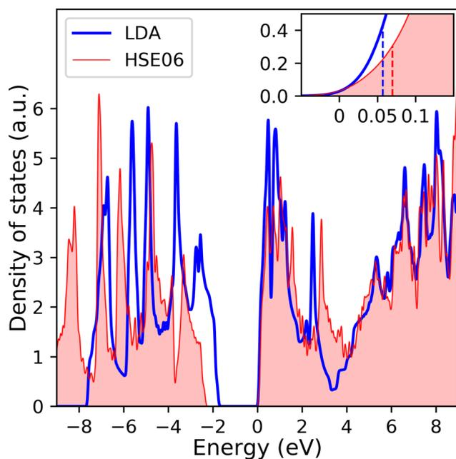
Fig. 2 Calculated electronic density of states of single-layer MoS<sub>2</sub> with LDA and HSE06 functionals. Zero energy level is set to the bottom of the conduction bands. The inset shows the zoom-in view of the region near the bottom of the conduction bands, in which the two vertical dashed lines, blue and red, represent the Fermi level at 1% doping for the case of LDA and HSE06 functionals parameter, respectively.
