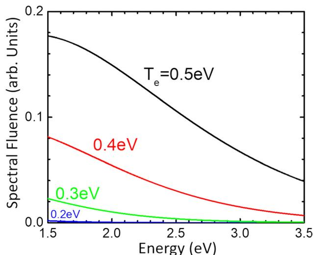
Fig. 7 The spectral fluence of doped monolayer MoS<sub>2</sub> at different electronic temperature. The values for other parameters are given in the text.
