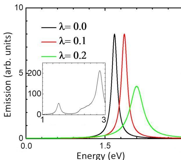
Fig. 5 The emission spectrum of monolayer MoS<sub>2</sub> at different values of  $\lambda$ . Inset: The corresponding absorption spectrum at  $\lambda = 0$ .
