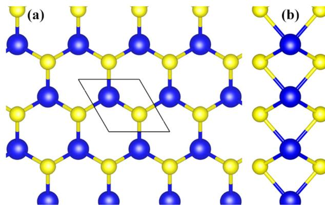
Fig. 1 Top view (a) and side view (b) of monolayer MoS<sub>2</sub>. Blue and yellow balls represent Mo and S atoms, respectively. The parallelogram in (a) indicate a unit cell of MoS<sub>2</sub>.
