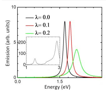
Fig. 5 The emission spectrum of monolayer MoS<sub>2</sub> at different values of  $\lambda$ . Inset: The corresponding absorption spectrum at  $\lambda = 0$ .
