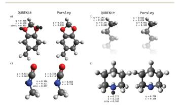
**Fig. 4** A comparison of selected force field parameters between QUBE (model **5b**), and Parsley. Charges on the atom centre and virtual sites (if applicable) are shown, along with the Lennard-Jones  $\varepsilon$  parameter (kcal mol<sup>-1</sup>).
