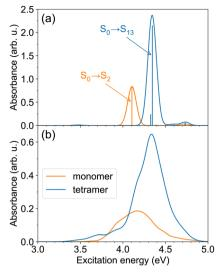
Fig. 2 (a) The  $\pi\pi^*$  absorption bands of the monomer and the tetramer, calculated with TD-ωB97X-D/def2-SV(P), for single model geometries. The monomer geometry was optimized at the B3LYP/def2-SV(P) level; the tetramer geometry (see Fig. 1a) was constructed from the optimized monomer geometry. (b) The  $\pi\pi^*$  absorption bands of the monomer and the tetramer at  $T \approx 300$  K. The spectra are obtained using TD- $\omega$ B97X-D/ def2-SV(P) calculations for 100 snapshots.
