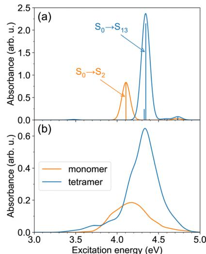
Fig. 2 (a) The  $\pi\pi^*$  absorption bands of the monomer and the tetramer, calculated with TD- $\omega$ B97X-D/def2-SV(P), for single model geometries. The monomer geometry was optimized at the B3LYP/def2-SV(P) level; the tetramer geometry (see Fig. 1a) was constructed from the optimized monomer geometry. (b) The  $\pi\pi^*$  absorption bands of the monomer and the tetramer at  $T \approx 300$  K. The spectra are obtained using TD- $\omega$ B97X-D/def2-SV(P) calculations for 100 snapshots.
