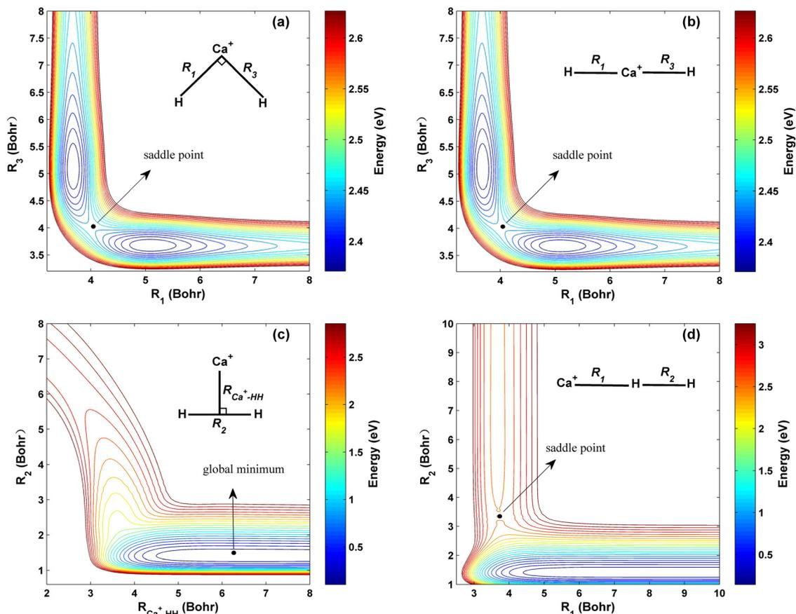
Fig. 3 Contour plots of the PIP-NN PES (a) for the bending angle between  $R_1$  and  $R_3$  fixed at  $90^\circ$ , (b) for the bending angle between  $R_1$  and  $R_3$  fixed at  $180^\circ$ , (c) for the  $C_{2v}$  symmetry and (d) for the  $\text{Ca}^+-\text{H}-\text{H}$  angle fixed at  $180^\circ$ .
