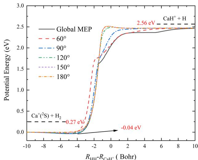
Fig. 4 Global MEP and the MEPs of the  $\text{Ca}^+(\text{}^2\text{S}) + \text{H}_2 \rightarrow \text{CaH}^+ + \text{H}$  reaction at five  $\text{Ca}^+-\text{H}-\text{H}$  angles ( $60^\circ$ ,  $90^\circ$ ,  $120^\circ$ ,  $150^\circ$  and  $180^\circ$ ) calculated on the PIP-NN PES.
