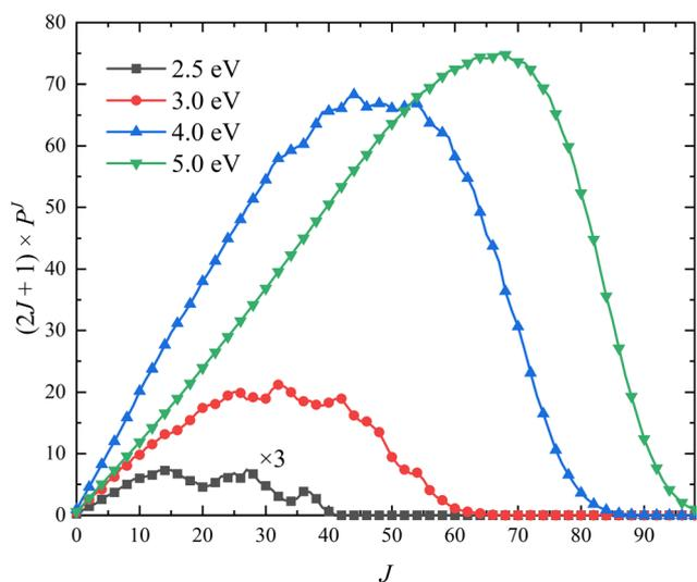
**Fig. 7** Opacity functions of the Ca<sup>+</sup>(<sup>2</sup>S) + H<sub>2</sub>(ν<sub>0</sub> = 0, j<sub>0</sub> = 0) → CaH<sup>+</sup> + H reaction at four collision energies (E<sub>c</sub> = 2.5, 3.0, 4.0 and 5.0 eV) calculated by the TDWP method on the PIP-NN PES.
