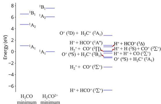
**Fig. 1** Excitation energies of  $\text{CH}_2\text{O}^{2+}$  and dissociation energies of the fragments which are possible. Results are obtained at the CCSD/cc-pVQZ level of theory. Excitation energies are shown at two geometries, the minimum of neutral formaldehyde (corresponding to vertical ionization) and the minimum of the ground state of the dication. These geometries are shown in Fig. S1 (ESI<sup>†</sup>).
