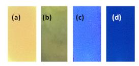
Fig. 8 Photographs of TLC plates, soaked in the solution of (a) HQCN and (b-d) after bubbling with hydrazine-contaminated air. Pictures taken after (b) 10 s (c) 60 s (d) 5 min.
