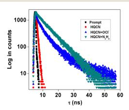
Fig. 5 Time-resolved fluorescence decay of HQCN (red), HQCN + OCl (blue), HQCN +  $N_2H_4$  (green) and prompt (black) ( $\lambda$  excitation = 370 nm). The calculated  $\tau$  was 0.7 ns ( $\chi^2$  = 1.21) for HQCN, 6.32 ns ( $\chi^2$  = 1.15) for  $HQCN + N_2H_4$  and 5.75 ns ( $\chi^2 = 1.09$ ) for  $HQCN + OCl^-$ .
