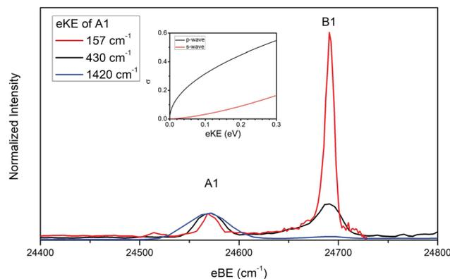
**Fig. 2** Cryo-SEVI spectra of  $\text{NiO}_2^-$  at three photon energies illustrating the differing signal attenuation for features A1 and B1 as eKE decreases. The intensity of each scan has been normalized to feature A1. Photon energies employed are 25 991 (blue), 25 001 (black), and 24 728  $\text{cm}^{-1}$  (red). Inset: photodetachment cross-section as a function of kinetic energy for s- and p-wave detachment as outlined by the Wigner threshold law.<sup>67</sup>
