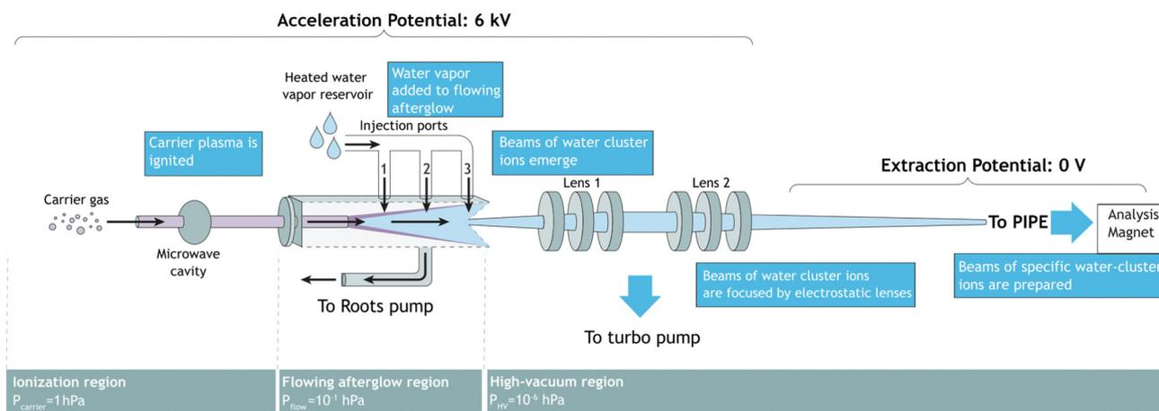
Fig. 1 Flowing afterglow ion source schematic. Three different conceptual regions are shown: the ionization region, the flowing afterglow region, and the high-vacuum region.
