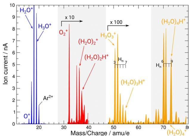
**Fig. 2** Mass spectrum of ion beams from the FLAGS in the regions featuring the relevant cationic species and protonated water clusters. The mass spectrum was produced using the cluster setting of the ion source (third column in Table 1). For clusters containing three and four oxygen atoms, a variety of clusters with a different number of H atoms are produced. Mass ranges with no water cluster signal ( $22\text{--}30 \text{ u e}^{-1}$  and  $38\text{--}48 \text{ u e}^{-1}$ ) are omitted.
