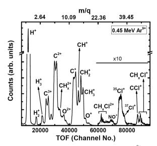
Fig. 2  $\,$  TOF spectrum (raw) of ions generated in 0.45 MeV  $\,$  Ar $^{9+}$  collisions with CH<sub>3</sub>Cl. Oxygenated species are originating from NO gas used in a trial run just before starting the experiments on CH<sub>3</sub>Cl.
