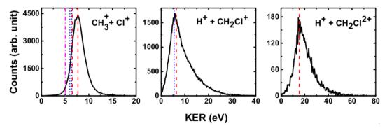
Fig. 4 Present experimental KER distributions (black curve) for the dissociation channels of  $CH_3Cl^{q+}$  (q=2,3) under 0.45 MeV  $Ar^{9+}$  along with our theoretical calculations (red dashed lines) and those reported in the literature: Duflot et al.<sup>23</sup> (blue dashed line), Walt et al.<sup>5</sup> (dashed dotted magenta line). See text for more details.
