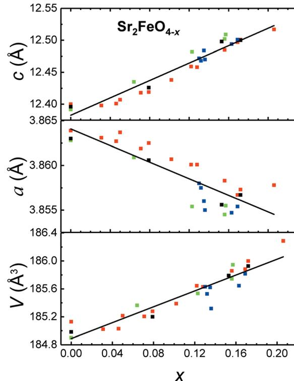
Fig. 6 Lattice parameters and volume per formula unit for  $\text{Sr}_2\text{FeO}_{4-x}$  as function of  $x$  as determined from XRD patterns at room temperature. The different colors correspond to different sample preparation series. The solid lines are linear fits to all data sets.
