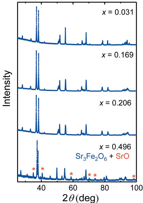
Fig. 5 Powder X-ray diffraction patterns of nominal  $\text{Sr}_2\text{FeO}_{4-x}$  samples with increasing oxygen deficiency  $x$ . The analysis of the PND pattern of the sample with  $x = 0.496$  revealed complete decomposition to  $\text{Sr}_3\text{Fe}_2\text{O}_6$  and  $\text{SrO}$ , where the peaks corresponding to  $\text{SrO}$  are marked by an asterisk.
