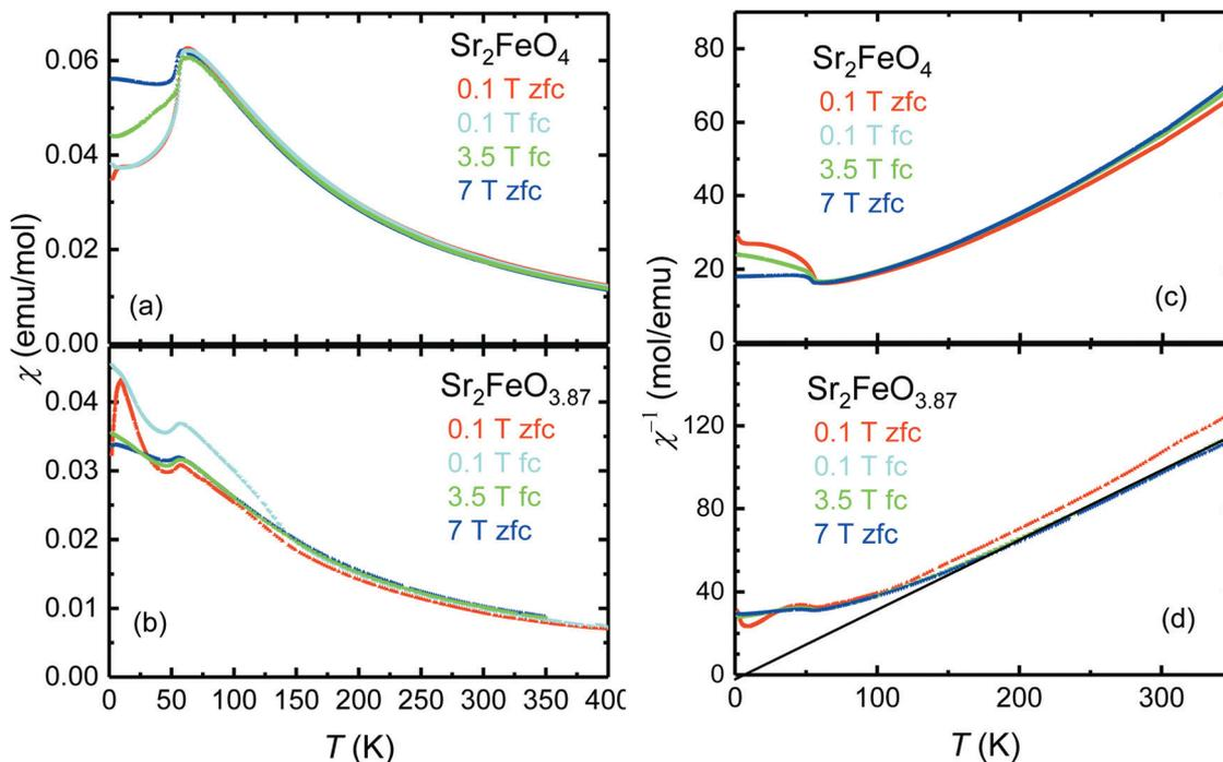
Fig. 7 Comparison of the magnetic susceptibilities  $\chi$  [(a), (b)] and inverse susceptibilities  $\chi^{-1}$  [(c), (d)] as a function of temperature of  $\text{Sr}_2\text{FeO}_4$  and  $\text{Sr}_2\text{FeO}_{3.87}$ .
