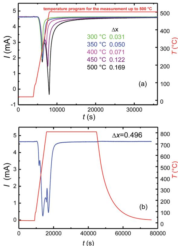
Fig. 3 Temperature programmed desorption curves for  $\text{Sr}_2\text{FeO}_{4-x}$  obtained by heating to the indicated temperatures. (a) Final temperature 300 to 500 °C, (b) final temperature 808 °C. The titration current  $I$  is represented as a function of time  $t$ . The temperature profiles for heating to 500 °C and to 808 °C are also shown. Typical sample masses were about 100 mg and the oxygen partial pressure was  $3 \times 10^{-6}$  bar.
