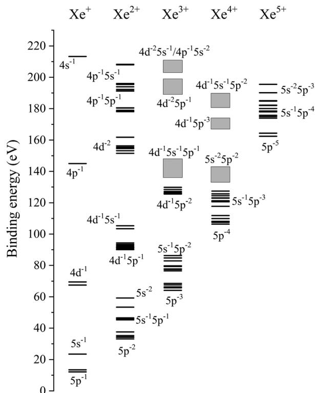
Fig. 3 Energy level diagram for the  $\text{Xe}^{2+}$  states ( $Z = 1-5$ ) lying below a binding energy of 220 eV. The energy levels for the  $4p^{-1}5l^{-1}$  states are from the present calculations, while the other levels shown with horizontal bars are from the literature.<sup>10,11,28</sup> Boxes indicate the binding energy ranges for the corresponding Auger structures observed in the 3d Auger decay.<sup>9</sup>
