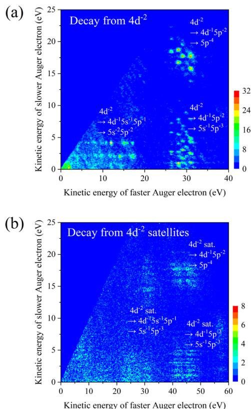
Fig. 6 Two-dimensional maps showing energy correlations between two Auger electrons emitted in the decay from (a)  $4d^{-2}$  and (b)  $4d^{-2}$  satellites, which are obtained from five-fold coincidences including the 4s photoelectron, CK electron and  $Xe^{4+}$  ion.
