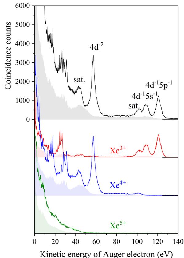
**Fig. 5** Auger spectra (solid line) coincident with 4s photoelectron, and spectra (shaded) delineating the background contribution. The black spectra on top are the replots of those in Fig. 4(a), and the other spectra are derived by further coincidence with product ions of  $Z = 3-5$ . The intensities of the spectra coincident with ions were corrected by the ion detection efficiencies. "sat." denotes correlated satellite structures analogue to Fig. 2.
