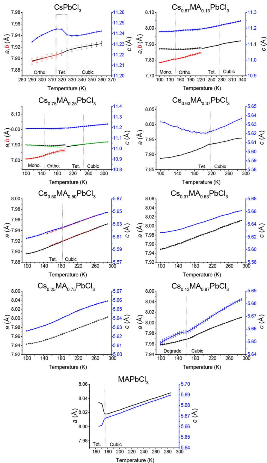
Fig. 8 Refined lattice parameter evolution (pseudocubic axes  $a$  black,  $c$  blue) elucidated from Pawley refinement of laboratory XRD data collected on the  $(\text{Cs}_x\text{MA}_{1-x})\text{PbCl}_3$  solid solution series. The cubic ( $Pm\bar{3}m$ ) to tetragonal ( $P4/mbm$ ) phase transformations in  $\text{Cs}^+$ -rich end of the series are dominated by second order effects.
