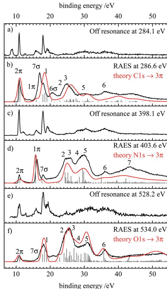
**Fig. 4** Resonant Auger electron spectra at the (b) carbon (d) nitrogen and (f) oxygen edge, as well as the corresponding off resonant measurements at each edge (a), (c) and (e). The computed spectra are shown in red and the contributions of individual final states are represented as grey sticks.
