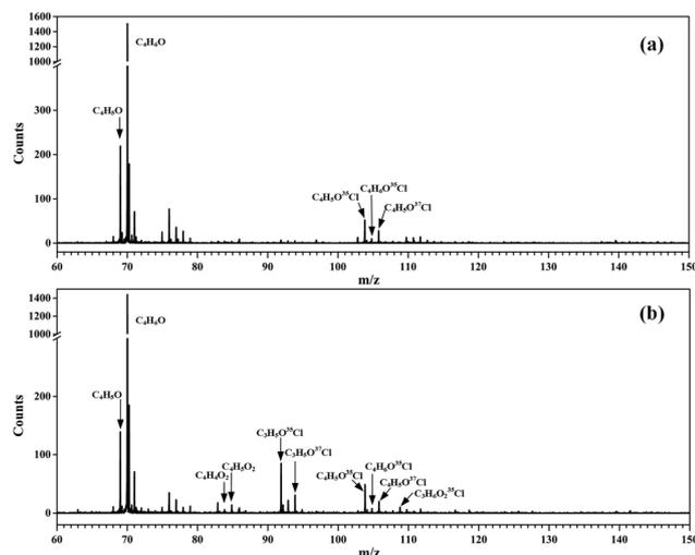
Fig. 1 Photoionization mass spectra acquired (a) without  $O_2$  and (b) adding  $O_2$  into the fast flow tube.
