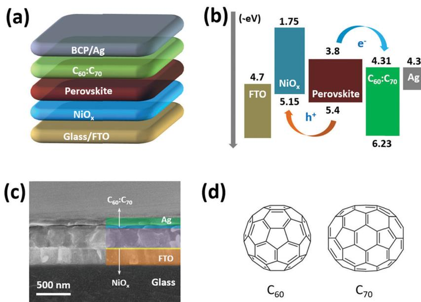
Fig. 1 (a) Schematic device structure of the PSCs; (b) schematic energy levels of the functional layers involved in the PSCs; (c) cross-sectional SEM image of a PSC; (d) molecular structures of  $\text{C}_{60}$  and  $\text{C}_{70}$ .
