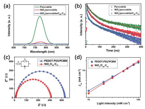
Fig. 4 PL (a) and time resolved PL (TR-PL) (b) spectra of bare perovskite,  $NiO_x/perovskite$  and  $NiO_x/perovskite/C_{60}$ : $C_{70}$  films; (c) EIS spectra of the PSCs using PEDOT:PSS/PCBM and  $NiO_x/C_{60}$ :  $C_{70}$  as the charge transport layers; and (d) light intensity dependence of  $J_{sc}$  for PSCs using PEDOT:PSS/PCBM and  $NiO_x/C_{60}$ :  $C_{70}$  as the charge transport layers.
