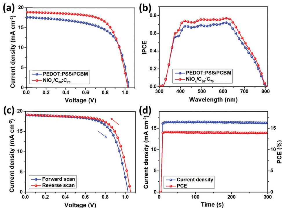
Fig. 2 Forward scanning  $J$ - $V$  characteristics (a) and IPCE spectra (b) of the PSCs using PEDOT:PSS/PCBM and  $\text{NiO}_x/\text{C}_{60}:\text{C}_{70}$  as the charge transport layers; (c) forward and reverse scanning  $J$ - $V$  characteristics of a best performing PSC using  $\text{NiO}_x$  and  $\text{C}_{60}:\text{C}_{70}$  as the HTL and ETL; and (d) current density and PCE as a function of time for the best performing PSC under a bias of 0.86 V.
