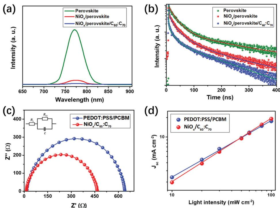
Fig. 4 PL (a) and time resolved PL (TR-PL) (b) spectra of bare perovskite,  $\text{NiO}_x/\text{perovskite}$  and  $\text{NiO}_x/\text{perovskite}/\text{C}_{60}:\text{C}_{70}$  films; (c) EIS spectra of the PSCs using PEDOT:PSS/PCBM and  $\text{NiO}_x/\text{C}_{60}:\text{C}_{70}$  as the charge transport layers; and (d) light intensity dependence of  $J_{\text{sc}}$  for PSCs using PEDOT:PSS/PCBM and  $\text{NiO}_x/\text{C}_{60}:\text{C}_{70}$  as the charge transport layers.
