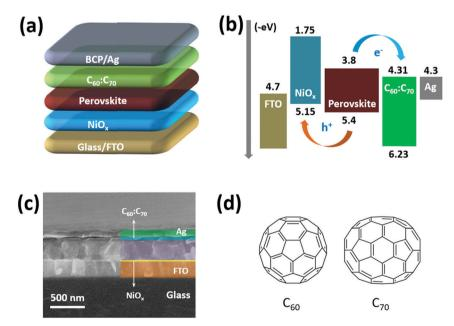
Fig. 1 (a) Schematic device structure of the PSCs; (b) schematic energy levels of the functional layers involved in the PSCs; (c) cross-sectional SEM image of a PSC; (d) molecular structures of  $C_{60}$  and  $C_{70}$
