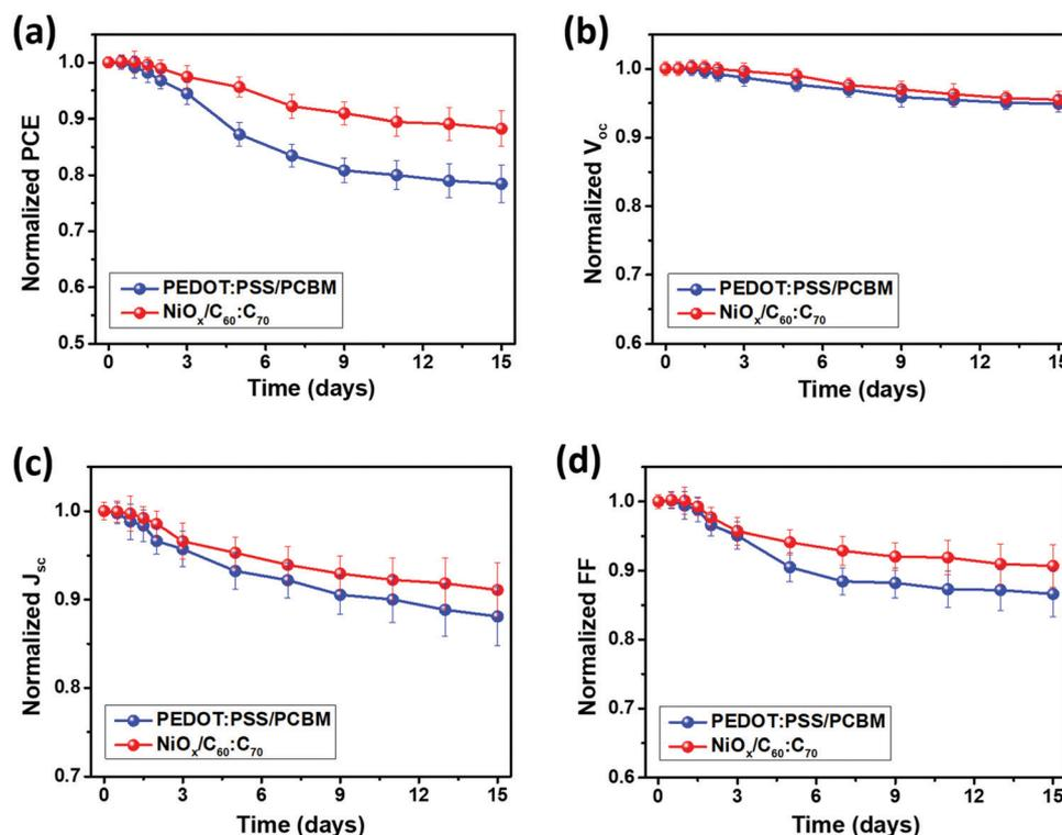
Fig. 5 Long-term stability of the PSCs using PEDOT:PSS/PCBM and NiO<sub>x</sub>/C<sub>60</sub>:C<sub>70</sub> as the charge transport layers, in terms of their normalized PCE (a), V<sub>oc</sub> (b), J<sub>sc</sub> (c) and FF (d) as a function of time.
