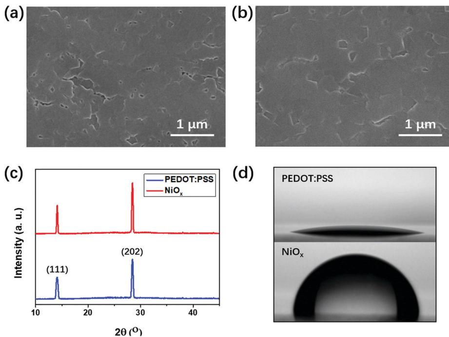
Fig. 3 SEM images of the  $(\text{BA})_2(\text{MA})_3\text{Pb}_4\text{I}_{13}$  perovskite films formed on (a) PEDOT:PSS and (b)  $\text{NiO}_x$ ; (c) XRD patterns of the perovskite films formed on PEDOT:PSS and  $\text{NiO}_x$ ; and (d) contact angles of water drops on the surfaces of PEDOT:PSS and  $\text{NiO}_x$  films.
